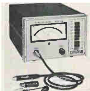
Solid state r-f millivoltmeter model 92A offers a basic accuracy of 1% of reading plus 1% of full scale. It measures 100 \mu v to 3 v from 10 khz to 1.2 Ghz in 8 ranges by convenient pushbutton selection. It has true rms response up to 30 mv (up to 3 v with proper accessory). A linear d-c output is provided. Price is $750. Boonton Electronics Corp., Parsippany, N.J. 07054 [367]
