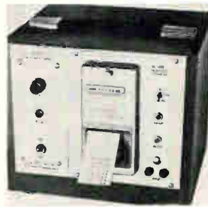
General purpose printing counter 22408 offers a counting speed of 10 pulses per second. Print-out periods of 1 every minute or 1 every 6 minutes can be selected by a panel switch. The counter can be made to print out totals accumulatively, or, reset to zero after each print-out. It features modular construction. Price is $500. Stoelting Co., 424 N. Hoeman Ave., Chicago 60624 [3871]
