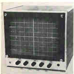
X-Y display oscilloscope model 101 is for all types of swept frequency and other measurements. It has a bright 11-in. screen marked with 2-cm squares for easy clear viewing. High sensitivity, variable from 5 mv/cm to 50 v/cm is another feature. Unit measures 11 x 9 x 11 \frac{1}{4} in., weighs 16 lbs. Price is $395. Telonic Industries Inc., P.O. Box 277, Laguna Beach, Calif. [365]
