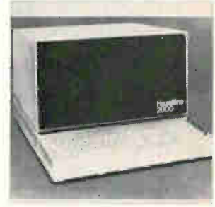
Desk-top crt display terminal model 2000 is fully interactive with a computer and completely compatible with existing programs and programing practices. It features a flicker-free 1,998 character display, and offers both split screen and highly flexible editing capabilities, including character and line insertion and deletion. Hazeltine Corp., Little Neck, N.Y. 11362 [3841]
