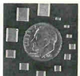
Monolithic ceramic chip capacitors feature an end metalization process that eliminates open circuits resulting from silver leaching or scavenging common in conventional end termination systems. Capacitance range is 10 to 330,000 pf and 10 to 5,600 pf in the BX and NPO dielectrics, respectively. Union Carbide Corp., Components Dept., P.O. Box 5928, Greenville, S.C. 29606 [348]
