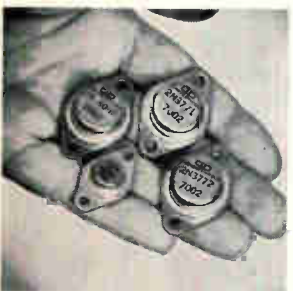
Single diffused mesa silicon npn power transistors now include the TO-66 package. Features include: V_{CBO} rating to 140 v, and I_C of 4 amps (typically) at 25°C, with a power capability of 30 w. Peak collector currents range from 3 to 7 amps. A unit price of 84 cents each in 100-999 lots is offered for the 2N3054 transistor. Power Physics Corp., Box 626, Eatontown, N.J. [440]
