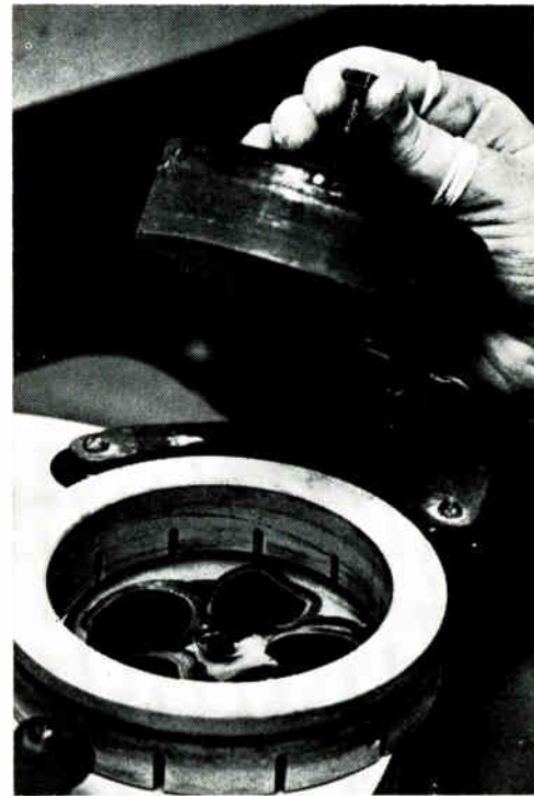
Headed for market. Fixture in which Bell & Howell polishes gallium arsenide wafers.
