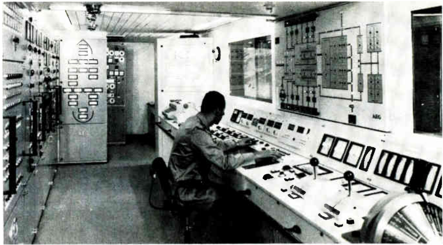
Out in the cold. Polar-Ecuador-class ship uses programable Telefunken data processors to control engines and refrigeration equipment.
