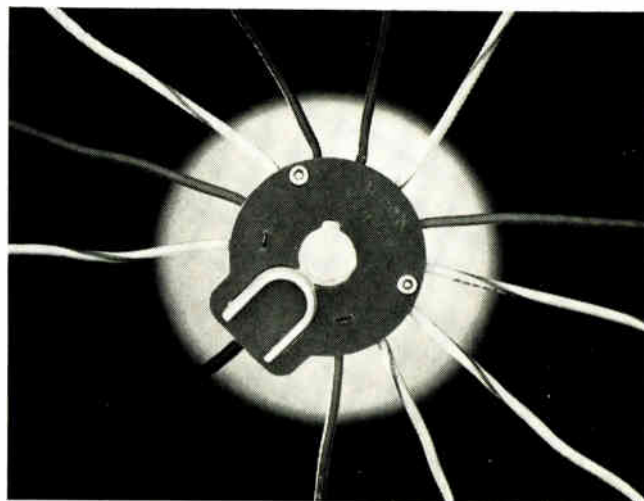
1. Safer socket. This picture tube socket has a high-voltage backing made of arc- and track-resistant laminate qualified to pass UL's flame resistance test.
