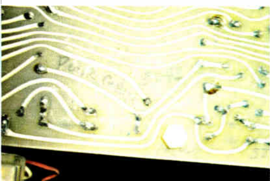
1. Poor parts. Some manufacturers sell hospitals less than top-flight equipment. Above, leaking electrolyte from faulty capacitor shorts resistor in a monitor. Below is board that failed but is in ECG machine anyway.
