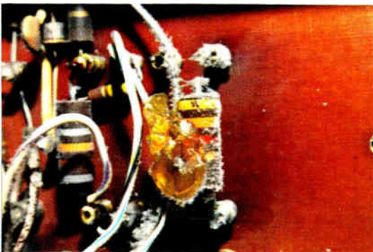
1. Poor parts. Some manufacturers sell hospitals less than top-flight equipment. Above, leaking electrolyte from faulty capacitor shorts resistor in a monitor. Below is board that failed but is in ECG machine anyway.
