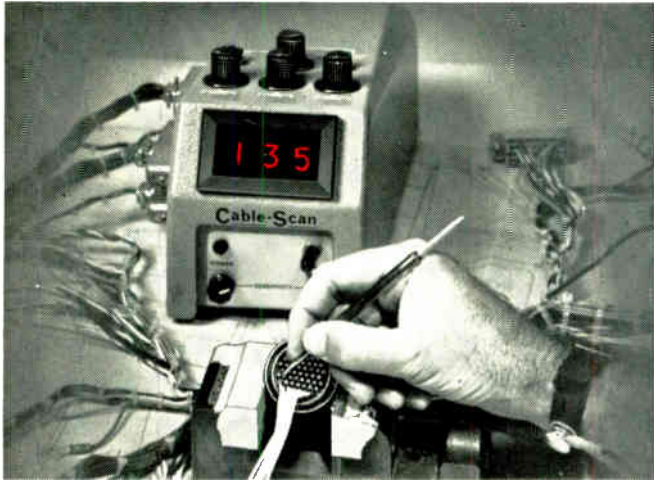
1 Quickly locate termination point by touching connector pin
