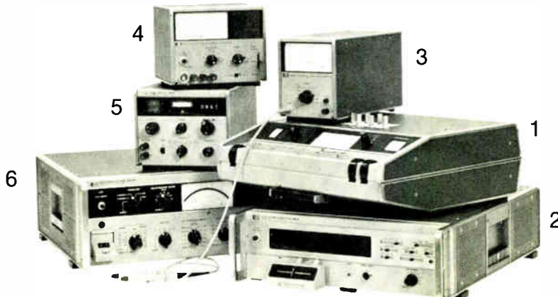
No. 1: 4342A Q Meter. No. 2: 4270A Automatic Capacitance Bridge. No. 3: 4328A Milliohmmer. No. 4: 4329A High Resistance Meter. No. 5: 4260A Universal Bridge. No. 6: 4470A Transistor Noise Analyzer.
