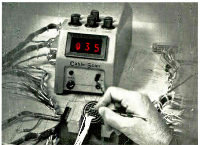
4 Complete installation and get immediate verification of proper termination
