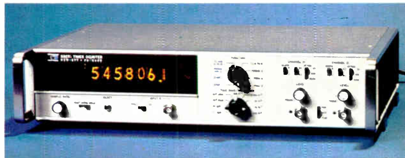
6. At work. Above, a 550-MHz binary and 400 MHz divide-by-5 quinary mounted in printed circuits to perform a decade function. Below, the packaged instrument, with frequency ranges of 0-50 MHz and 0-550 MHz.
