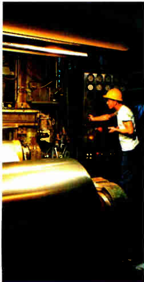
Measuring current, voltage and roll forces to control product uniformity.
