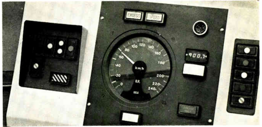
Prototype. Light-emitting diodes form rays, showing maximum permissible speed, around dial and form number display, showing distance to next speed change.
