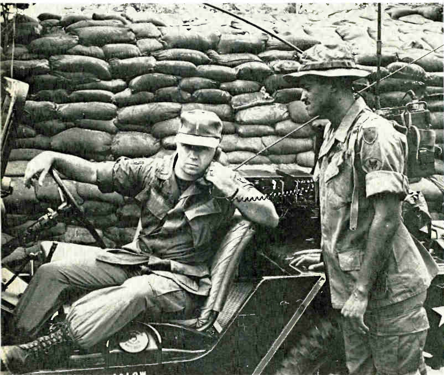
1. Combat veterans. Army radios that get out to where the action is most often are the AN/PRC-77 manpack and the jeep-mounted AN/GRC-163. Both can operate in a voice-secure mode, using an AN/KY-28 digital scrambler.
