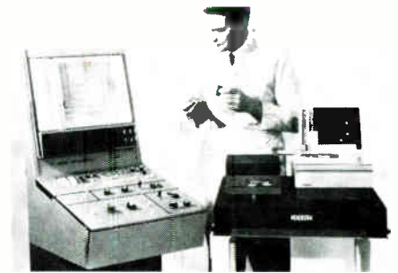
The Gould Micro-Topographer™ 200 recording (below) of a micro electronic circuit illustrates the potential of this analytical tool for micro surface geometry.
