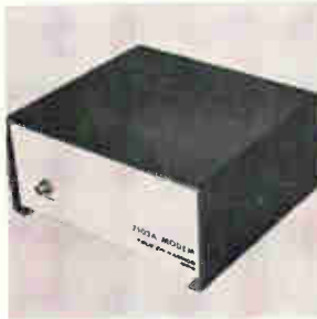
Data set type 7103 provides full-duplex asynchronous digital transmission at rates to 300 baud on standard voice-grade telephone lines. It is interchangeable with the Bell System 103 data set. It is available in three modes: originate-only, answer-only, and automatic selection for originate or answer operation. Tele-Dynamics Div. of AMBAC Industries Inc., Ft. Washington, Pa. [382]
