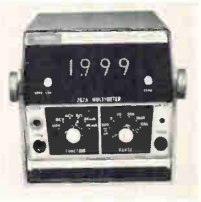
Digital multimeter model 262A has available 25 ranges for measuring d-c voltage and current, a-c voltage and current, and ohms. It has a basic d-c accuracy of 0.1% of reading. All the d-c ranges feature automatic polarity indication; and automatic zero correction circuitry assures maximum stability. Price is $375. United Systems Corp., 918 Woodley Rd., Dayton, Ohio 45403 [362]
