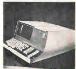
The Datapoint 2200, referred to as an "intelligent terminal", offers keyboard entry, video display, dual magnetic tape cassette unit for both program and data storage, automatic Bell System compatible communication capability, and general purpose computing. The desk-top unit features a crt display. Computer Terminal Corp., 9725 Data Point Dr., San Antonio, Texas [384]
