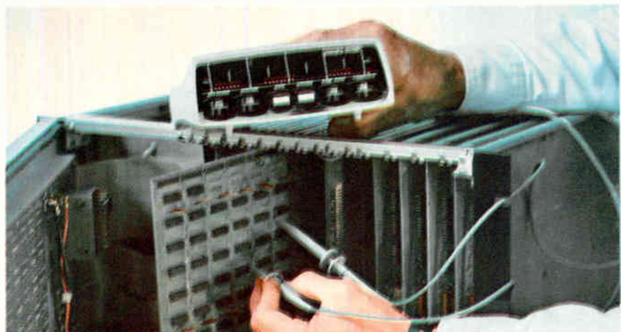
Tight check. Tester monitors digital performance. Unit's light-emitting diodes display 1s and 0s of pulses, and stores them.
