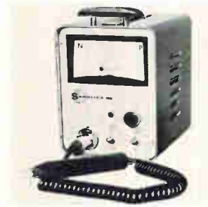
Portable tester model H-720 identifies silicon and germanium semiconductor materials as N or P types, with fast swing needle readout. Readouts are achieved with minimal probe pressure especially suitable for use on very thin substrate. The long-life probe pins are easily replaced when required. Unit measures 8½ x 6 x 8 in. Semimetals Inc., 172 Spruce St., Westbury, N.Y. 11590 [363]
