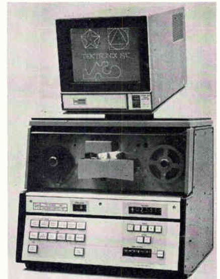
First step. Tektronix Inc. is entering N/C field with a two-axis ($9,750) and three-axis ($11,000) model for both point-to-point and contouring machines. Position and command registers operate in binary code, so they can be used in computer-directed systems being planned. Prices do not include type 611 storage display ($2,695) that provides quick check for any gross errors in programming.
