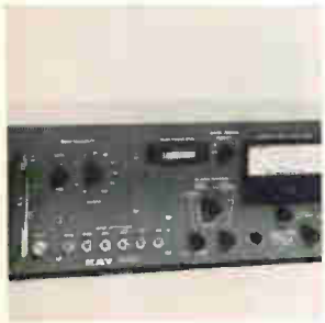
Automatic noise figure meter model 792A1 features a 75 ohm, 10 to 250 Mhz tuned amplifier input and a 75 ohm, 10 to 1000 Mhz full range noise head. A direct-reading panel meter provides noise figure readings over a range of 0 to 20 db for the 6-db automatic reference; 3 to 30 db for gas tube and solid state sources. Kay Elemetrics Corp., Pine Brook, N.J. 07056 [361]
