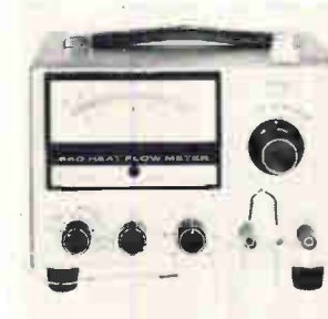
Heat flow meter model 860 offers 10% accurate measurements from -300° to +400° F. Measurements are repeatable to within \pm 2% at any temperature on all ranges except the two most sensitive where repeatability is limited by meter noise. Rise time is less than 1 sec on all ranges except the most sensitive where it is 3 sec. Keithley Instruments Inc., Aurora Rd., Cleveland [367]
