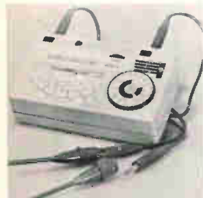
Taut-band multimeter model N-2 has 41 ranges. D-c voltages range from 0.012 to 600 v full scale. A-c voltages range from 1.5 to 600 v. These are flat to 100 khz. D-c current ranges are from 30 \mu a to 6 amps f-s. A-c current ranges cover 150 \mu a to 6 amps. Resistance, db level and temperature are also measured. Medistor Instrument Co., N. Northlake Way, Seattle, Wash. [365]
