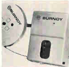
Automatic terminal machine model TFM installs vinyl-insulated, nylon-insulated or uninsulated terminals mounted on low-cost Mylar tape. It is foot-pedal actuated and crimps between 1,500 and 2,000 terminals per hour. No die changing is required as the die assemblies are rotated on turntables to accept varied terminal sizes and types. Burndy Corp., Norwalk, Conn. 06852. [422]
