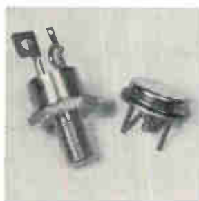
Silicon planar power transistor SDT9650 has usable h_{FE} at 200 amps, V_{CE0} up to 300 v, saturation voltage at 200 amps less than 1 v, and I_{CBO} less than 100 \mu\text{a} at 150 v V_{0B} . Units are available in a TO-68 and TO-114 package. Typical applications include high current control circuits, converters and inverters. Solitron Devices Inc., Blue Heron Blvd., Riviera Beach, Fla. [442]
