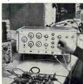
Pulse generator model 8010A is actually two pulse generators with a common output. Each channel’s pulse shaping controls (width, amplitude, risetime, fall-time, offset) are controllable independently, giving an infinite variety of complex waveforms when the waveforms are combined in a common output. Hewlett-Packard Co., 1501 Page Mill Rd., Palo Alto, Calif. [362]
