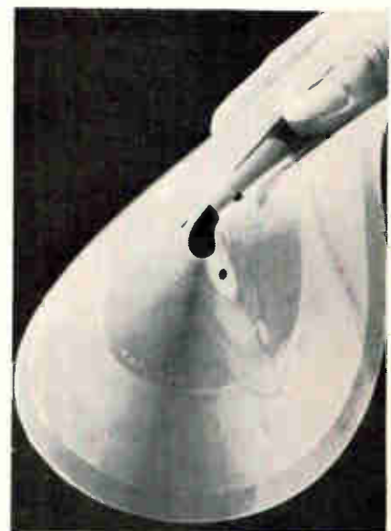
. . . set. Flexible disk rotates at 1,500 rpm, riding an air cushion, and generates one frame per turn.
