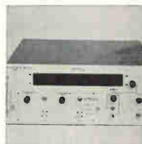
Time interval meter model 536 provides a highly accurate measurement of time with a resolution and accuracy of 1 nsec, thus allowing resolution down to ½ foot at velocities equaling or approaching the speed of light. It is suited for use in high resolution radar ranging, radar altimeters, radar and laser measurements, etc. Nano Fast, 410 W. Erie St., Chicago 60610 [364]
