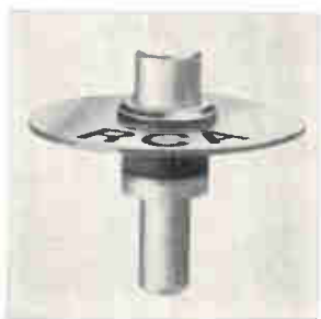
Silicon npn transistor 2N5920 features the overlay multiple-emitter-site construction. It is intended for solid state equipment for microwave communications, S-band telemetry, microwave relay link, phased-array radar, and distance measuring equipment. It offers 2-w output with 10-db gain at 2 Ghz; 3-w with 12-db gain at 1 Ghz. RCA, Somerville, N.J. [441]
