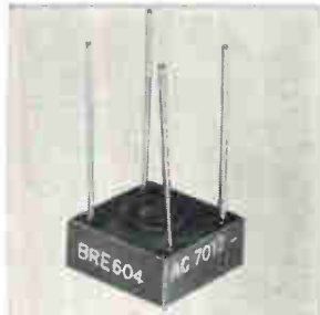
Silicon, single-phase bridges series BRE600 feature 6 amps average output at a temperature coefficient of 55^{\circ}\text{C} . Peak reverse voltages are 50 to 800 v. Peak surge rating (1 cycle) is 50 amps. Packaging is accomplished with a 0.6 \times 0.6 \times 0.25 in. case, base mounted by either through bolt or a \frac{3}{8} in. 6-32 stud. Rectifier Components Corp., 124 Albany Ave., Freeport, N.Y. [437]
