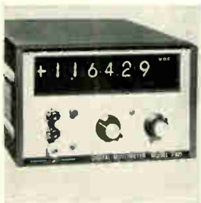
Digital voltmeter/multimeter model 7005 features a 5½-digit readout, 10-microvolt resolution, and an accuracy of \pm 0.005\% . Measurements can be made at a rate up to 5 samples per second, and readings include an auto-positioned decimal point, polarity sign, and annunciator. Base price is $1,295. Systron-Donner Corp., 888 Galindo St., Concord, Calif. 94520 [361]
