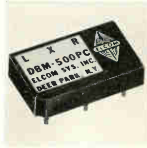
Low profile, double balanced mixer model DBM-500 PC occupies 0.08 cu in. and is designed to plug into a 14-pin dual-in-line socket or mount directly to a p-c board. It has an r-f and l-o input range of 2 to 500 Mhz, and an i-f that operates from d-c to 500 Mhz. Unit contains matched, low noise Schottky barrier diodes. Elcom Systems Inc., West Industry Court, Deer Park, N.Y. [403]
