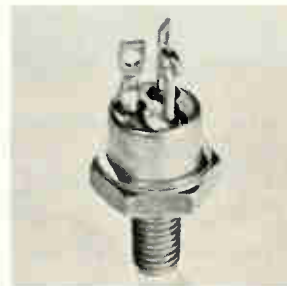
R-f power transistors series 2N-2877, 2N2878, 2N2879 and 2N2880 are rated at 30 w with a beta cutoff up to 50 Mhz, with collector-to-emitter voltage of 80 v. Applications include high frequency inverters, converters, linear amplifiers, and high speed switching regulated power supplies. General Semiconductor Industries Inc., 230 W. 5th St., Tempe, Ariz. [443]
