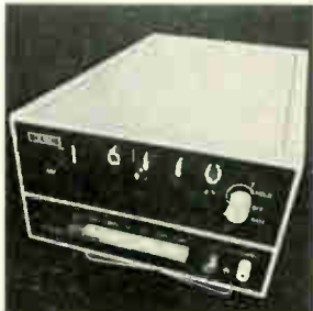
Digital integrating microvoltmeter DS-100 solves instrument drift and repeatability problems suffered by aerospace and industrial technicians involved in physical measurements and other low level instrumentation. Zero drift due to time and temperature is stopped with the Auto-Zero method of a-d conversion. Doric Scientific Corp., 7601 Convoy Court, San Diego, Calif. [367]
