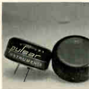
Light controlled, variable resistor called Pi-Switch provides a solid state isolation switch. The CSN 756 is rated at 0.75 w and 600 v; and CSN253, rated at 0.25 w and 350 v. Units feature current capability to 10 ma in the light source element, and a dynamic range of 200 to 10^6 ohms in the resistance element. Pulsar Instruments Inc., Hurlingame Ave., Redwood City, Calif. [342]
