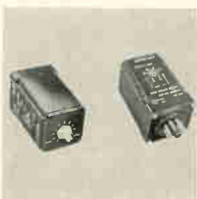
Inexpensive, octal base, plug-in time delay relay known as Sensitak model 41 uses a solid state timing module. The timer is of the "on delay" type. When voltage is applied to the control circuit, the timer contacts transfer only after a preset time delay, and then return to normal after power is removed. Price (1-24) is $19.80. Struthers-Dunn Inc., Pitman, N.J. 08071 [347]
