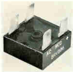
Six-ampere silicon single phase bridges designated the BRV600 series have been value engineered to those rectifying applications that require surge ratings of 50 amps or less. Voltage types from 50 to 1,500 v are featured, with packaging in a 0.4 in. case having fast disconnect appliance type terminals. Rectifier Components Corp., 124 Albany Ave., Freeport, N.Y. [441]
