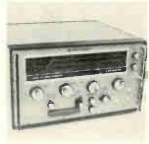
Sweep generator model 103 covers, without plug-ins, a frequency range from 10 Mhz to 12,400 Mhz. Range is divided into 3 bands (0.01-4.2 Ghz, 4.2-8 Ghz, 8-12.4 Ghz), selected by a front panel control. Continuous sweep is up to 4,200 Mhz. Output power is 2 mw minimum to 8 Ghz, 20 mw minimum above that level within \pm 0.5 db. Space-Kom Inc., P.O. Box 10, Goleta, Calif. [404]
