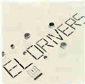
Solid state switches series EL20, EL200 are designed and specified as drivers for electroluminescent displays. They have forward and reverse blocking voltages from 200 to 400 v with high reverse gain for minimum power consumption, and can be driven directly from low-level IC's. Price (100-999) is from $1.85 each. Unitrode Corp., 580 Pleasant St., Watertown, Mass. 02172 [437]
