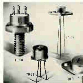
Power transistors KS6101 through KS6130 range from 20 v to 100 v. They switch currents from 0.25 amp to 20 amps. Typical turn-on and turn-off times for any of these currents are 35 nsec and 85 nsec, respectively. Packages range from TO-39 for low currents to TO-3 for currents above 5 amps. Kertron Inc., 7516 Central Industrial Dr., Riviera Beach, Fla. [439]
