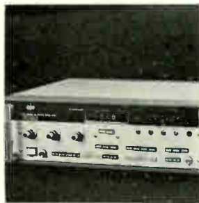
Sampling digital voltmeter model 1166 measures true root-mean-square or peak of continuous or bursts of complex waveforms. It employs a square law detector that measures waveform over an interval as short as 10 \mu sec with a sample period of 3.3 msec, making it suitable for computer controlled measurements. Scientific Atlanta Inc., P.O. Box 13654, Atlanta, Ga. 30324 [362]
