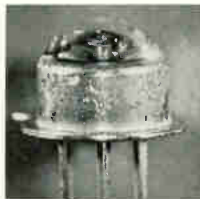
Npn type phototransistor model BP101 is for use in automatic electronic flashlight units, electronic toys and similar applications. It is packaged in a TO-18 case with the light falling through a translucent epoxy cover. It features a typical photo current of 150 \mu a for an illumination of 1000 Lux. Siemens Corp., 186 Wood Ave., South Iselin, N.J. 08830 [442]
