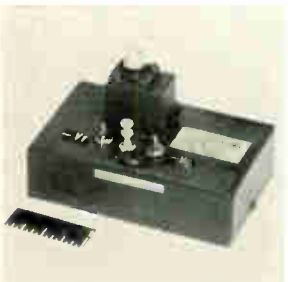
Voltage-tuned, transferred-electron oscillator S293, a solid state replacement for klystrons, operates at 10 Ghz. It can be tuned throughout a 6% bandwidth centered at 10 Ghz, and a minimum power output of 10 mw. Unit makes use of a differential negative resistance in the bulk of a GaAs diode. Price (1-10) is $700 each. RCA Microwave Solid-State, Harrison, N.J. 07029 [405]
