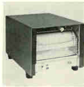
Pen recorder model 310 has a full scale span of 1 mv to 100 v, accuracy better than ½%, pen response up to 10 in. per sec, and single or dual chart speeds of ¼ in. per hr to 6 in. per sec. Four-inch fan-fold paper offers a quick-reference feature. All electronics are on an easily replaceable p-c board. Laboratory Data Control Inc., 42 Shelter Rock Rd., Danbury, Conn. [363]
