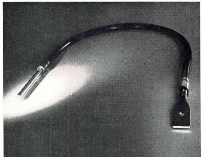
Provide input-output geometry conversions such as round-to-square, round-to-slit, etc.
