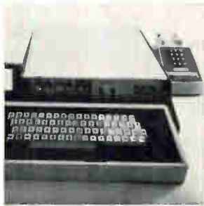
Full-scale crt terminal called Envoy weighs 30 lbs and is packaged in a rugged carrying case. It displays up to 1,024 alphanumeric characters on a 5-in. diagonal crt. Compatible with teletypewriter data communication systems, it transmits and receives data over telephone lines at a rate of either 10 or 30 characters per sec. Applied Digital Data Systems Inc., Hauppauge, N.Y. [406]
