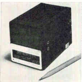
Dual-output tracking power supply LXN-3-152 is designed to power operational amplifiers. It features tracking accuracy of 0.1% absolute voltage difference for all conditions of line, load and temperature. Regulation is 0.1%, line or load. Ripple is 1.5 mv rms, 5 mv peak-to-peak. Temperature range is 0 to 71°C. Lambda Electronics Corp., Broad Hollow Rd., Melville, N.Y. [385]
