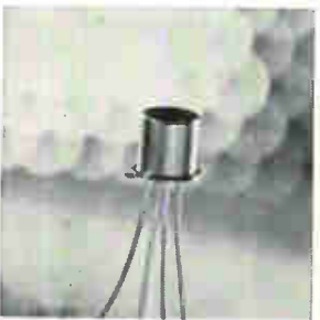
P-channel, insulated gate MOS FET 3N174 features low leakage and high input impedance, important in minimizing drift in operational amplifiers and in providing high accuracy in electrometer circuits. At 25° C maximum drain current is -5 na; maximum gate-terminal current, -2.5 pa; low threshold voltage, -2 to -6 v. Texas Instruments Inc., P.O. Box 5012, M/S306, Dallas [441]
