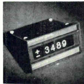
Bidirectional counter model MDBC Mini-Diget will count incoming positive pulses at a rate exceeding 15 Mhz and, with proper signal applied, add or subtract these pulses to arrive at a net accumulation. Provisions within the unit enable the user to preset to an arbitrary count of zero before initiating new count. Instrument Displays Inc., 18 Granite St., Haverhill, Mass. [367]
