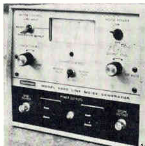
Line noise generator 3020 serves a dual purpose. It generates a controlled line transient similar to rectifier or scr noise on the a-c line, as well as measuring line noise up to 1 kv peak. Noise amplitude and position are continuously adjustable and a sweep mode is provided for scanning noise pulse over 360°. Beckman Instruments Inc., Harbor Blvd., Fullerton, Calif. [362]
