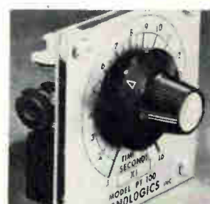
Solid state panel timer PT-100 has adjustable timing ranges from 100 msec to 1,600 sec. Accuracy is \pm 2\% with repeatability to \pm 1\% at constant temperature. Maximum time for reset is 50 msec. Operating ranges are from 12 v to 110 v, a-c or d-c, and four mounting options are available. Price (small lots) is under $25. Chronologics Inc., 24 Martin St., Webster, N.Y. [4241]
