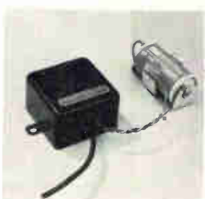
Battery-powered, thermocouple-to-current converter TA-01 offers integral cold junction compensation. The thermocouple amplifier amplifies a 5-mv full scale signal (120° C) into a 100 \mu a output signal with an accuracy better than 1%. Load impedances up to 10 kilohms can be driven by the output circuit. Price is $50. Integrated Controls Inc., Box 17296, San Diego, Calif. [4281]
