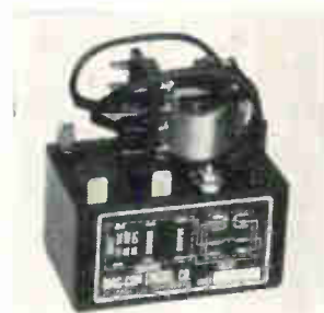
Resistance sensing power relay uses electrodes to detect the level of water, chemicals, or slurries in a storage tank. It can also operate as an ice bank control or condensation detector in protective control systems. Units come with either a 40 kilohm or 500 kilohm trip point. Output relay is rated at 8 amps. Mag-Con Engineering Co., 85 Richardson St. S.E., St. Paul, Minn. [4221]
