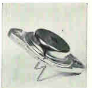
H-v npn silicon power transistors now come as 700 v devices in production lots. Specifications include: saturation voltage less than 600 mv at 3 amps; sustaining V_{CEO} in excess of 500 v; and minimum h_{FE} at 3 amps of 15. Typical uses include vertical and horizontal deflection circuits for crt instrumentation. Solttron Devices Inc., Blue Heron Blvd., Riviera Beach, Fla. [443]
