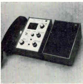
Vhf/f-m solid state maritime receiver MR-201 consists of a 25-w unit in a rugged splash-proof case, a control panel, speaker panel and a handset. It uses only one crystal in a stabilized master oscillator, permitting immediate use of all 55 of the new maritime channels. It provides rapid channel selection through digital tuning. Collins Radio Co., Dallas 75207 [381]
