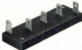
5A — Type 3KBH5 10A — Type 3KBH Two thru-holes for mounting #8 screw Body: 3" L x 1" W x 5/16" H
