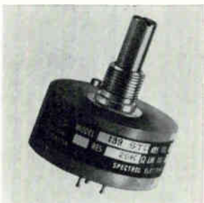
Single-turn, cermet precision pot model 139 features a high-power rating suited for industrial use in controls and instrumentation. It offers a resistance range of 500 ohms to 1 megohm, essentially infinite resolution, and a standard independent linearity of \pm 0.5\% . Power rating is 5 watts at 40^\circ C. Spectrol Electronics Corp., 17070 E. Gale Ave., City of Industry, Calif. [426]
