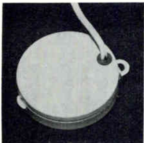
Micro water detector is designed to detect water on surface of the walls, ceilings, standpipes, and areas where space is limited and access difficult. When water contacts the cartridge, it swells up, pressing against an internal water-proof switch which starts alarm. Unit can be connected into existing alarm systems. Price is $21.95. Retawmatic Corp., 509 Fifth Ave., New York [425]
