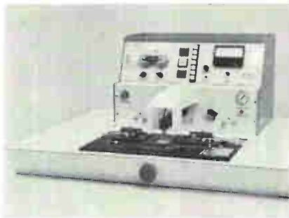
Step-by-step. Production-line tool can trim all resistors on a substrate. Step-and-repeat mechanism is at front.
