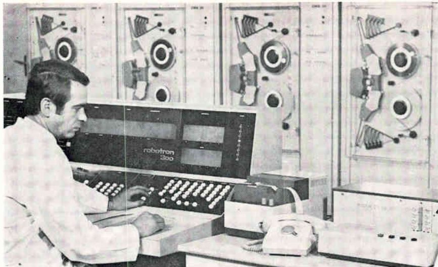
At the console. The most powerful computer in East Germany's stable is the Robotron R300, here linked with a 200-baud data transmission terminal.
