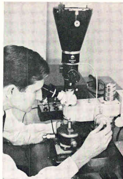
Surfacing. Microscope system measures smoothness with high precision.
