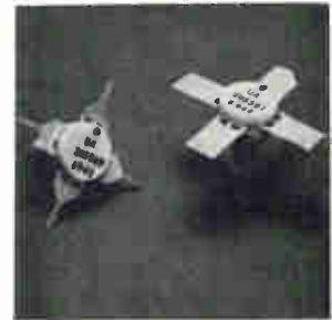
Silicon power transistors models 2N5589, 2N5590 and 2N5591 have been optimized for operation at 13.6 v for f-m/vhf mobile communications equipment. The devices, featuring low inductance TO-71 and TO-72 stripline packages, provide 3, 10 and 25 watts, respectively. Price (1-99) ranges from $7 to $24 each. Electronic Components Division, United Aircraft, Trevose, Pa. 19047 [439]
