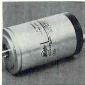
Size 18 d-c tachometer CVO 9612 001, for industrial applications, features a high output of 100 v per 1,000 rpm and exhibits low-ripple voltage. Used for feedback-drive or velocity servo-drive functions, it serves as an integral part of a contour-control system. Ambient temperature range is -54^\circ to +100^\circ C. Singer-General Precision Inc., Kearfott Division, Little Falls, N.J. [423]
