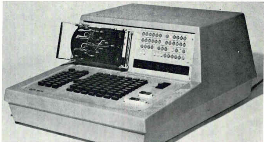
Patchwork. Combining digital modules, Ceta Electronics operational computer achieves its speed by using prediction algorithms to vary increments.
