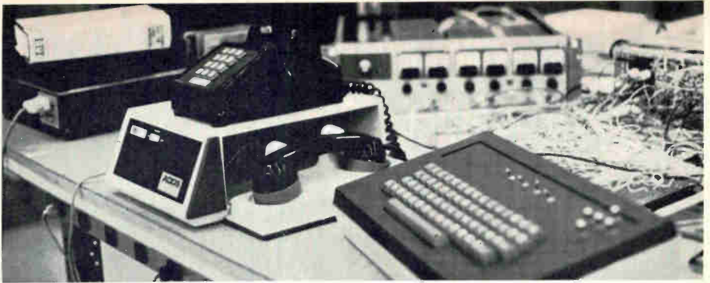
Data by phone. The acoustic coupler is seen under test in the laboratory; a telephone is seated on top of the coupler while a keyboard is used to punch in the desired information.
