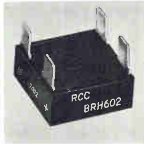
Silicon single phase bridges BRH/T300 and BRH/T600 are 3- and 6-amp bridges for high reliability industrial and military use. They feature a miniature thermally matched design (1 x 1 x 0.4 in.). Both series have 10 to 2,500 v types with respective single cycle surge current ratings of 50 and 125 amps peak. Rectifier Components Corp., 124 Albany Ave., Freeport, N.Y. [438]
