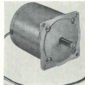
Slo-Syn synchronous/stepping motor type LS50 has a low shaft speed of 28.8 rpm at 60 hertz without step-down gearing. Used as an a-c motor it will start, stop, and reverse almost instantly. The motor will stop within 25 msec without external braking. It is rated for 120 v 0.2 amp. It features 40 oz-in. torque. Superior Electric Co., 382 Middle St., Bristol, Conn. 06010 [424]
