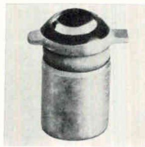
Phototransistors type OP300 will generate light currents in excess of 12 ma at irradiance of 1 mw/cm 2 . With normal light input, the current output is sufficient to function as an IC-logic circuit driver. Units are built in a package that may be mounted on 0.087-in. centers and are suited for IBM system 3 minicard uses. Optron Inc., 1201 Tappan Circle, Carrollton, Texas [438]
