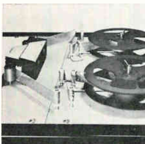
Paper tape spooler accommodates 5-8-track paper or mylar tape at bidirectional speeds to 1,000 characters/sec and rewind speeds to 1,000 characters/sec. The high reliability and ruggedness is suited for numerical control, ground support systems, test equipment, digital data handling, and computer input. Datascan Inc., 1111 Paulison Ave., Clifton, N.J. 07013 [405]
