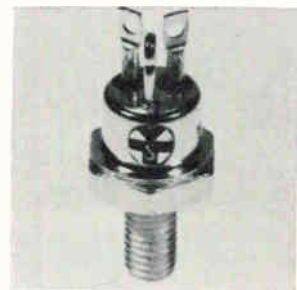
Power transistors JAN 2N2880 and JAN TX 2N2880 are npn silicon triple-diffused devices for power amplifiers and switching uses. Features include: 30 w dissipation capability, low leakage current, 20 Mhz minimum gain cutoff, and low drive requirements. Units are suited for use in h-f inverters and converters. Silicon Transistor Corp., East Gate Blvd., Garden City, N.Y. [443]
