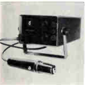
Rotary thermal wire stripper model RT-1 features centrifugal-force insulation severing that ends conductor damage. It will strip most insulations used in electronics manufacturing including Teflon and Kapton without damage to even hair-like No. 40 strands. Wire diameters are No. 40 to 0.300 in. Roto-Therm Division, Republic Corp., 950 N. Sepulveda Blvd., El Segundo, Calif. [425]
