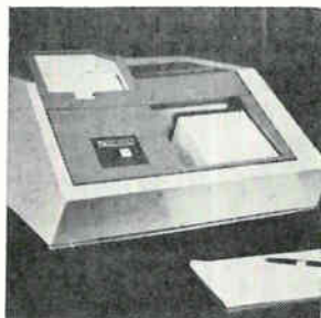
Card reader SR-600 maintains a rate of 600 80-column cards each minute or 750 51-column cards each minute. As an intermediate speed card reader, it comes as a table unit offering simplicity of operation. Unit weighs 125 lbs, has a hopper capacity of 1,400 cards and a stacker capacity of 1,000 cards. Data Products Corp., 6219 DeSoto Ave., Woodland Hills, Calif. [406]
