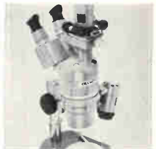
Hybrid-circuit production and inspection time is cut 50% by a new stereo-microscope system. The Infoscope projects circuit diagrams, waveforms or digital displays into the bonding operator's or inspector's field of vision. This permits checking assembly accuracy and performance without looking away from the eyepieces. Olympus Corp of America, Nevada Dr., New Hyde Park, N.Y. [428]
