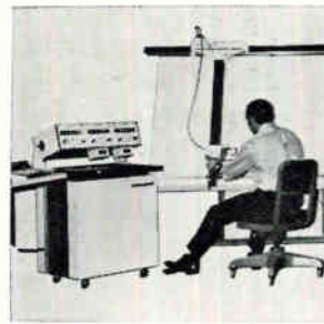
Auto-trol digitizer model 3800 converts graphic data to digital form for input to computer programs. Precise x and y coordinate values are recorded by operator command onto punch cards, paper tape, magnetic tape, or computer terminals in operator-wired formats compatible with customers' computer program. Auto-trol Corp., 6621 W. 56th Ave., Arvada, Colo. 80002 [403]
