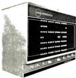
System-oriented computer model A includes 4,096 16-bit words of core memory, 32,768 words of disk memory, a memory access controller, a central processor, an input/output bus, and a teletypewriter with paper tape reader and punch. The 32,768-word disk is field expandable to 65,536 or 131,072 words. Price is $14,995. Multidata, 15142 Goldenwest Circle, Westminster, Calif. [426]
