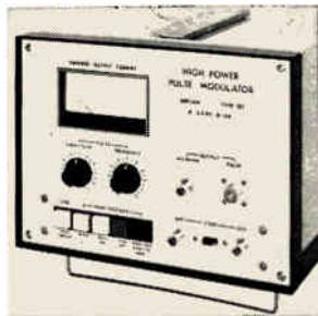
Pulse modulators are computer-controllable for automated testing. Type 101 provides up to 10 kw of regulated and continuously variable peak power output in a compact design. Standard units are available with peak outputs of 3.5 kv at 3 amps, 5 kv at 2 amps, and 100 v at 100 amps. Price is $985; delivery, 2 weeks. Bertan Associates Inc., 15 Newtown Rd., Plainview, N.Y. [362]
