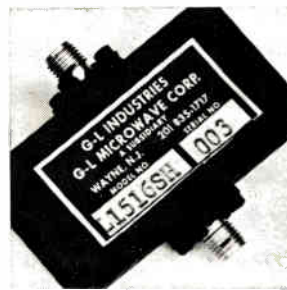
High power diode limiter for sensitive receiver protection can withstand 5 kw of peak power, with pulse lengths up to 250 \mu sec. It operates in the 1,400 to 2,300 Mhz band. Insertion loss is 0.25 db maximum; spike leakage, less than 0.12 erg; flat leakage, 40 mw. Recovery time is less than 1 \mu sec, and vswr is 1.20 max. G-L Microwave Corp., Wayne, N.J. 07470 [407]
