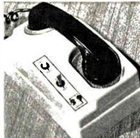
Acoustic data coupler Design 79 offers a method of communicating with a time-shared computer or with another remote data terminal via an ordinary telephone. The telephone handset is simply placed on the data coupler, the coupler attached to a teletypewriter or other data terminal, and the computer number dialed. Design Elements Inc., 2074 Arlington Ave., Columbus, Ohio [423]
