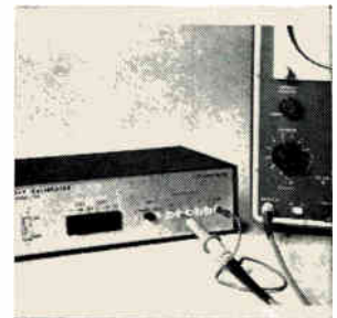
X-Y calibrator model 132, for oscilloscopes and volt ohmmeters, provides accurate d-c or square wave output up to 1 Mhz and from 0.10 through 10 v. Precision time base calibration with 0.005% accuracy is provided by crystal oscillator and IC dividers. It measures 3 x 11 x 6 in. Price is $99.50 in kit form or $198.50 assembled and tested. Paramatron Corp., Rochester, N.Y. [368]
