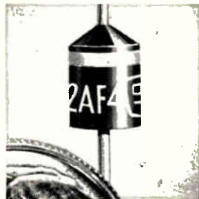
Plastic encased silicon rectifiers series 2AF4 have a d-c rating of 2 amps, resistive or inductive load, at 25° C and are available in 6 different piv ratings from 100 to 1,000 v d-c. Maximum rms input voltages range from 70 to 700 v d-c. All are designed to sustain peak 1 cycle surge currents of up to 60 amps. Sarkes Tarzian Inc., 415 N. College Ave., Bloomington, Ind. [442]
