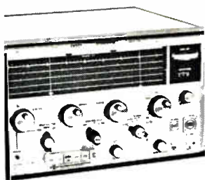
Sweep generator series 101 generates swept frequency signals from 0.1 to 24 Ghz without external plug-in units. Range is divided into 5 bands, selected by a front panel control: 0.1 to 4.2 Ghz, 4.2 to 8.2 Ghz, 8.2 to 12.4 Ghz, 12.4 to 16.4 Ghz and 16.4 to 24 Ghz. Continuous sweep is up to 4100 Mhz including 100 Mhz to 4200 Mhz range. Space Kom Inc., Box 10, Goleta, Calif. [401]
