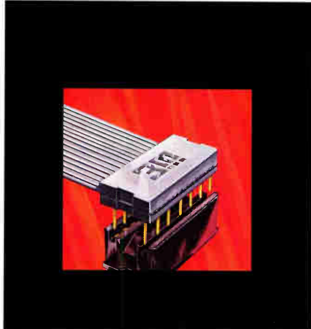
Dual In-Line plug Transitions. 14 and 16 position DIP plugs transition between round conductor flat cable on .050" centers to I.C. Socket patterns. Pins are located on .100" x .300" grid.
