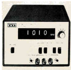
Autoranging digital dbm/khz test set 1101A is for telecommunications circuits. It combines the capability for both frequency and transmission level measurements. It provides direct digital readout for signals between -50 dbm and +10 dbm; 10 readings per sec at a resolution of 1hz. Price is $1,185. Telecommunications Technology Inc., 920 Commercial St., Palo Alto, Calif. [365]
