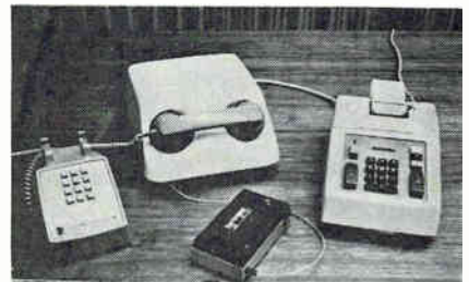
Tieup. Terminal for computer input consists of adding machine, cassette recorder, and acoustic coupler.
