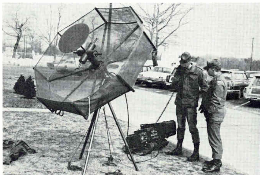
Mighty mite. Three GI's can carry the 120-pound uhf satellite terminal. The Collins-built TRC-156 puts 20 watts into its 5-foot dish.
