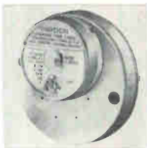
Synchronous hysteresis, heavy-duty gear head motor MA20 provides an output torque of 15 pound inches for speeds of 1/60 rpm to 14 days per revolution. It is available with optional size output shaft, anti-backlash gear train, and voltage range of 24, 120 and 240. Motor is custom built to meet exact OEM needs. General Time Corp., Route 8, Torrington, Conn. 06790 [342]
