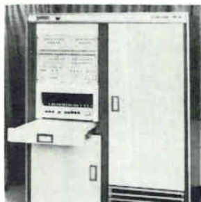
Simultaneous data communications between 120 remote terminals and a central computer over a single voice grade line is possible with the Dyne-Com 70 multiplexer. With a synchronous line efficiency of over 80%, it can handle 6 or 7 times as many terminals as conventional time division multiplexers. Prices start at $60,000. Dynelec Systems Corp., Glen Rock, N.J. [385]
