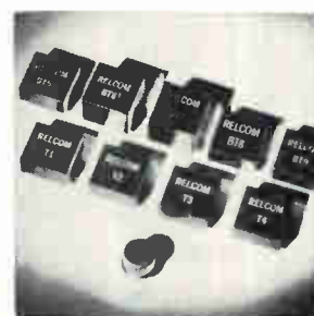
Miniature transformers feature a frequency range of 0.1 to 700 Mhz and have insertion loss of less than 0.5 db. Impedance transformations include 50 ohms to 12.5, 25, 50, 100, 200, and 800 ohms. Six transformers are balanced with both amplitude and phase balance specified. Four units are single ended Relcom, Charleston Rd., Mtn. View, Calif. [347]
