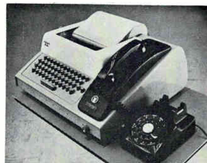
Conversion. Coupler on right side of Teletype transforms it into terminal.
