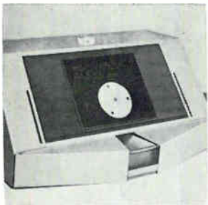
Optoline assembly director uses fiber optics to provide visual instruction to the operator in the positioning of printed-circuit board components. Components are selected from a rotating tray, and a central member indexes the power source current through a program module to the visual fiber optic readout panel. Hollis Engineering Inc., Nashua, N. H. 03060 [421]
