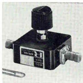
Continuously variable coaxial attenuators come in tiny packages. In both narrow and broad bandwidths, the units are available for frequencies from 2 to 12.4 Ghz. Typical maximum vswr's range from 1.5 for narrowband (20% bandwidth) units to about 2 for octave bandwidths. Power rating for all units is 6 watts, average. Solitron/Microwave, 37-11 47th Ave., L.I.C., N.Y. [402]
