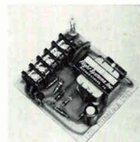
Interface unit 114A converts line voltage command signals to TTL or DTL logic levels. It performs the direct interface between IC logic and machine tool control circuit. Immunity to false actuation in either the "1" or "0" state is incorporated. Unit will not actuate on any noise signal up to 3 msec duration. Price (1-10) is $19.50. Flight Systems Inc., Mechanicsburg, Pa. [388]
