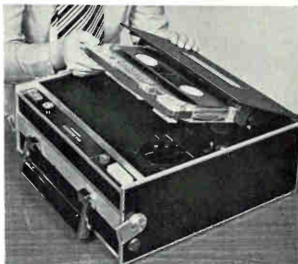
Outside. The magazine, the size of a large book, drops into recorder. The reels can be removed for operation on reel-to-reel machines.
