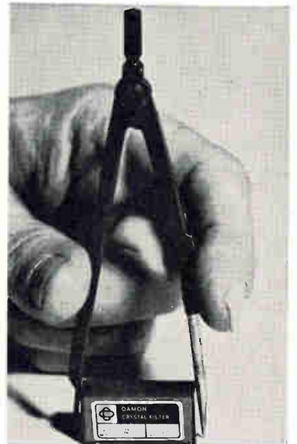
Spacesaver. Wideband IC filter measures 1.25-x-0.625-x-0.35 inch.
