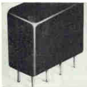
Half-size microminiature, crystal-can relays require only 100 mw pull-in. The 2pdt series is rated at 2 amps and meets MIL-R-5757E electrical requirements, while surpassing the environmental requirements. Units withstand vibration of 20 g to 2,000 hz, acceleration of 100 g minimum, and 50 g shock. Welch Relay Co., 11161 W. Pico Blvd., Los Angeles [341]
