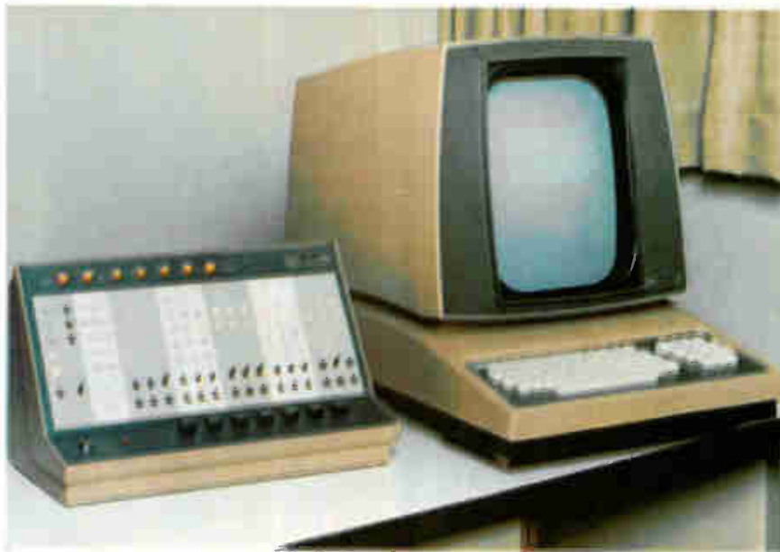
Companion. To use the computer capabilities of the PDS-1 to best advantage, a separate control console, shown at left, is required.
