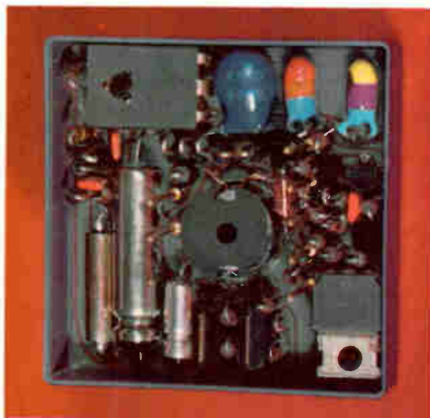
Powermite. Source for integrated circuits takes up less than 2 cubic inches. It is thin enough to permit half-inch spacing of printed-circuit boards, yet puts out 5 watts to power any of the families of digital logic.
