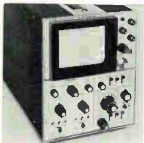
High frequency, dual channel oscilloscope 1050 offers a triggering device that eliminates trace flicker. Another advantage is maintenance of signal synchronization regardless of the vertical positioning of either trace. Unit also features sensitivity to 1 mv/cm from d-c to 25 Mhz in both channels with X10 gain. Dumont Oscilloscope Laboratories Inc., W. Caldwell, N.J. [367]
