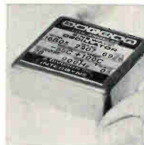
Sine wave tuning fork oscillator model 16B05's output is a short-circuit protected sine wave featuring a maximum harmonic wave form distortion of only 5%. Frequency may be specified from 360 hz to 15 khz. Input voltage is 22 to 32 v d-c with current dependent upon frequency (25 to 35 ma). Price is $148 in 100 quantity. Barden Co., 2217 Purdue Ave., Los Angeles [383]
