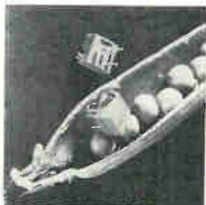
Center-tap 3/8-inch trimmer potentiometer model 75SCT features resistance values from 100 ohms to 20 kilohms and stand-offs for easy board washing. Its diallyl phthalate case is impervious to all normal cleaning solvents. An "O" ring seals the adjustment shaft to protect internal parts against severe environments. Techno-Components, 7803 Leona Ave., Van Nuys, Calif. [347]
