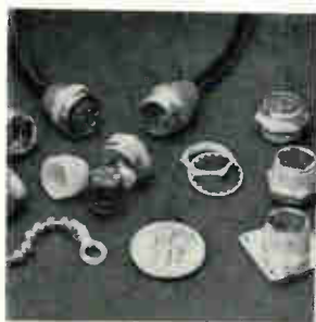
Miniature multipin connectors feature a 7/16-28 threaded coupling. With 5 key mechanical polarization one shell size of ½ in. max. o-d is available in 3, 5, 7, and 9 power contacts and in combinations of coax and power types. All are rated at 1 amp. Insulating materials are fused glass or molded thermosetting compound. Ted Mfg. Corp., Shawnee Mission, Kan. [341]
