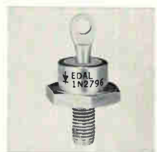
Silicon power rectifiers come in stud mounted DO-5 packages. A double diffused, passivated junction technique assures stable electrical characteristics. Both standard and bulk avalanche types in voltage ratings from 50 to 1,000 piv are available. The F3, F4 and F5 series offer max. forward current of 31, 37 and 50 amps, respectively. Edal Industries Inc., East Haven, Conn. [439]
