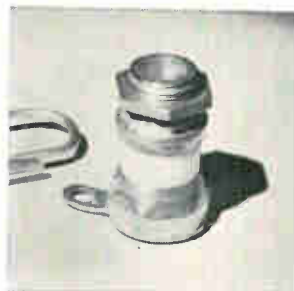
Alumina insulated bushing assembly AB1 provides electrical isolation for variable air dielectric trimmer capacitors mounted on conductive chassis or other surfaces. It has a resistance rating of 10 6 megohms, and can be used with any standard air trimmer with a 15/64 in.-64 threaded bushing. Price in lots of 100 is $2 each. Voltronics Corp., West St., Hanover, N.J. [343]
