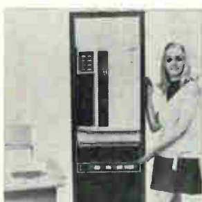
An IBM-compatible magnetic tape system with controller, interface, and software for the PDP-8 computer, is available. Computer access is by a 3-cycle data break facility with a transfer rate of 10 K, 12-bit words/sec at a tape speed of 24 ips. A single 2400-ft tape reel will store in excess of 100 million bits. Computer Equipment Corp., 3707 Rawlins, Dallas 75219 [427]
