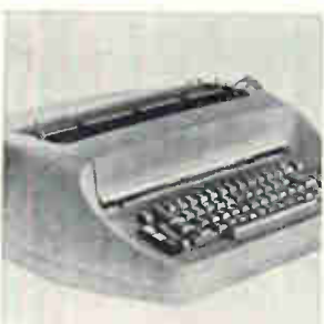
Portable communications terminal Edityper is designed to operate in a conversational mode. Designed for the computer time-share market, the terminal will transmit and receive the EBCDIC, or correspondence, code. The terminal will operate with a Bell series 103A or F data set, or an equivalent acoustic coupler. Epsco Inc., Providence Highway, Westwood, Mass. 02090 [426]
