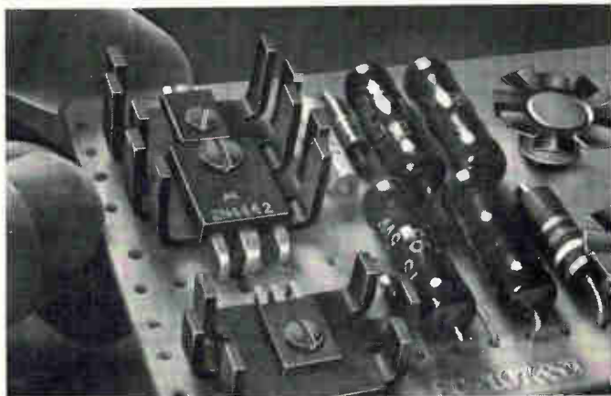
Power levels of plastic power devices such as X58's, MS9's, and M386's can be increased up to 80% in natural convection and 500% in forced air when used with PA and PB Dissipators. PA's need only .65 sq. in. to mount; PB's 1.17 sq. in. Staggered finger design gives these light-weight dissipators their high efficiency.
