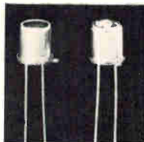
Photodiode detectors MD1 and MD2 are designed to complement the company's light-emitting semiconductors. Responses range from 0.4 to 1.1 microns. At 0.9 micron the MD1, which has built-in optics, has a minimum sensitivity of 1.5 \mu\text{a}/\text{mw}/\text{cm}^2 ; and the MD2, with its flat lens, a minimum sensitivity of 3 \mu\text{a}/\text{mw}/\text{cm}^2 . Monsanto Co., 10131 Bubb Rd., Cupertino, Calif. [442]
