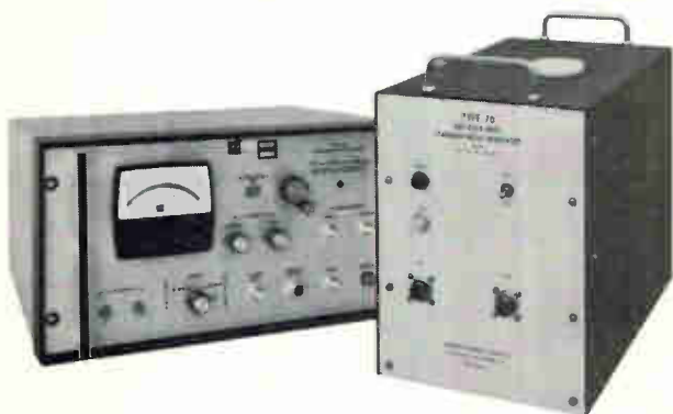
AIL's precision pair: Type 136 Precision Test Receiver (left) is priced at $1350; Type 07009 DC to 9 GHz Hot/Cold Standard Noise Generator at $1950.
