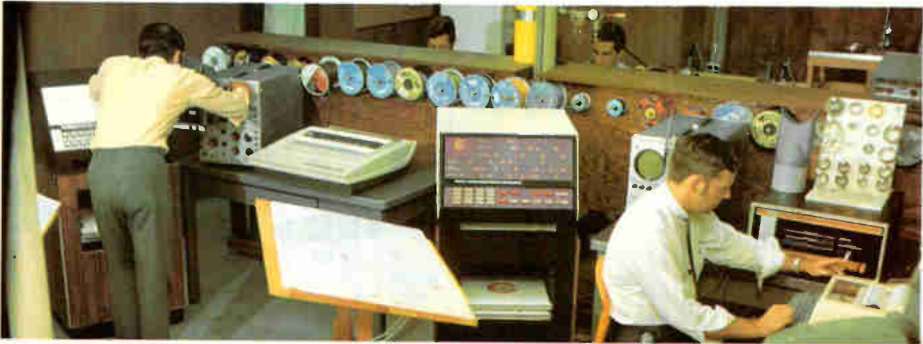
Team member. Disk memory, center, has an input-output section that makes it compatible with most computers.
