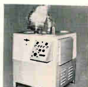
Automated wafer finishing machine simultaneously flat finishes both sides of silicon wafers, ceramic substrates and many other materials with surface finishes to one micron precision. One worker operating several machines can easily achieve production rates exceeding 1,000 high-precision 1-in. wafers or substrates an hour. P.R. Hoffman Co., 359 Cherry St. Carlisle, Pa. [424]
