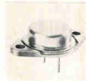
High-voltage epitaxial transistor type 1843 has a typical speed of 30 Mhz at voltages up to 375 v and a peak current of 30 amps. It is for use in power supplies, voltage regulators, d-c to d-c inverters, linear amplifiers, d-c to a-c converters, and control circuitry. Price in 100 lots rated at 300 v is $45.75 each. Westinghouse Electric Corp., Box 868, Pittsburgh, Pa. [438]
