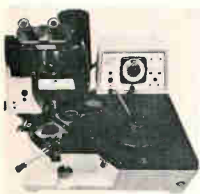
Optical mask alignment and exposure system model 500D offers operational flexibility and initial exposure rates as high as 430 wafers per hour. Wafer-to-mask alignment is accomplished by an X-Y joystick control. The system's vacuum chuck will accommodate wafers from 0.750 to 2.125 inches in diameter. Electroglas Inc., 150 Constitution Drive, Menlo Park, Calif. 94025 [421]
