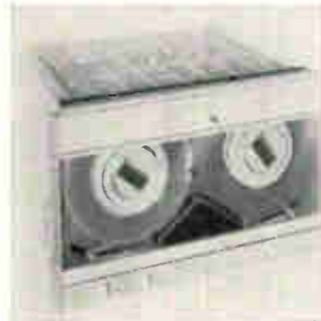
Magnetic tape handler model 3600 is for the small digital computer data acquisition, and data communication fields. It is IBM 360-compatible, sells at under $3,000, operates at 24 ips, handles 8½-in. reels and includes all read/write, servo and motion control electronics. It handles 800, 556, or 200 bpi, ½-in. wide tape. Digitronics Corp., Albertson, N.Y. [403]
