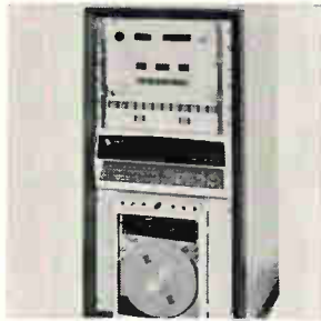
Computerized data logger model 100C makes it possible to monitor up to 100 analog points, translate into binary data and instantaneously produce finished computations in engineering units. The computer has a 4,096 word core memory, expandable up to 16,381 words. All software is provided from the factory. A. D. Data Systems Inc., Linden Ave., Rochester, N.Y. [406]
