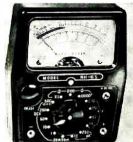
Multitester model NH-65 is a 21-range, 20,000 ohms/volt d-c unit that features a mirrored scale, safety diodes for overload protection, ultrasensitive 0.44 \mu a D'Arsonval movement, and an easily read 2-color scale. Unit uses 1% matched precision resistors. It measures 4 1/2 x 3 3/8 x 1 1/2 in., weighs less than 2 lbs. Mura Corp., 355 Great Neck Rd., Great Neck, N.Y. [364]
