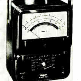
Ruggedly-built a-c current leakage tester model 229 offers a performance approximating the normal perception curve to within \pm 1 db and it will measure leakage currents as small as 5 \mu a. Ranges cover a-c current: 0-0.3, 1, 3 and 10 ma; and a-c voltage from 0 to 150 v. Accuracy is \pm 2\% at 60 hz. Price is $90. Simpson Electric Co., 5200 W. Kinzie St., Chicago 60644 [368]
