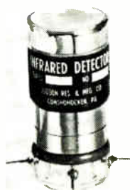
Infrared detectors series J-10 operate at liquid nitrogen temperature and cover the wavelength range from the visible through 5\frac{1}{2} microns. The photosensitive element is of single crystal indium antimonide. Sensitivities are available to 20 \times 10^{10} cm/w at 5 microns with time constants of less than 2 \mu sec. Judson Research and Mfg. Co., Conshohocken, Pa. 19428 [383]
