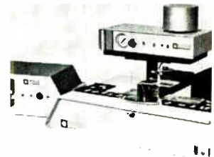
Semiautomatic air abrasive resistor trimmer for hybrid circuits operates on a 3 second prober/shuttle cycle. With a 1 second average trim time, the production rate of the model RA-650 is 900 units per hour. Accuracies of 0.5% or better over a range of 10 to 100,000 ohms can be obtained, depending on the measuring bridge. Axion Corp., 6 Commerce Park, Danbury, Conn. [424]
