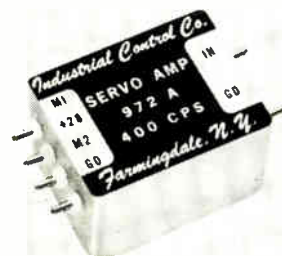
Servo amplifier 972A needs no external components, yet drives a 9-w, 400-hz servo motor. Size is 1 \times \frac{3}{4} \times \frac{5}{8} in. Transfer gain is X500, input impedance 20 kilohms, and required B+ only \pm 28 v, d-c unregulated. Heat sinking is through the base. The circuit is overload-protected and rfi-quiet. Price is $110 in lots of 1,000. Industrial Control Co., Farmingdale, N.Y. [386]
