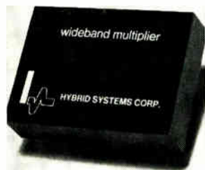
Wideband analog multiplier model 105 has 10 Mhz -3 db bandwidth and a 250 v/ \mu sec slew rate. It is capable of a full power response of 20 v peak-to-peak out to 4 Mhz. Accuracy is specified to be 1% for 4 quadrant operation. Unit is short circuit protected and suited for p-c mounting. Hybrid Systems Corp., 95 Terrace Hall Ave., Burlington, Mass. [385]
