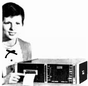
Multichannel data logger model DL-2 provides for automatic and precise measuring and recording. It is designed with a digital display and a printed record of up to 100 different electrical signals. Monitoring speed is normally one signal per second and intervals between scans can be adjusted up to 5 minutes duration. P/P/M Inc., 7016 Euclid Ave., Cleveland 44103. [425]
