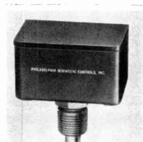
Mercury thermostats can be fixed set at any temperature between -20° and 200° F. Once calibrated, the unit will maintain the temperature to within 0.05° C over one year or 100,000 operations. It switches 2 amps a-c or d-c and comes with a plastic control housing and an aluminum or stainless steel probe. Philadelphia Scientific Controls Inc., 1135 Cedar Ave., Croydon, Pa. [345]
