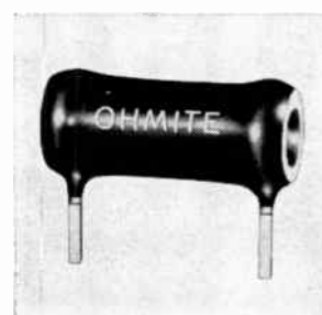
Radial-lead, power wirewound resistors designated PC-58 are available in 3-, 5-, and 8-watt sizes. By eliminating cutting, bending and forming leads, the PC-58 cuts labor costs up to 21.9% with productivity increases of 28.1%. Resistance range is 0.51 to 7,000 ohms. Price of the 3-w unit is 24 cents in lots of 500. Ohmite Mfg. Co., 3601 W. Howard St., Skokie, Ill. [342]
