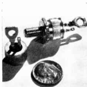
Twenty-five ampere triac thyristors SC60 (stud mounted) and SC61 (press fit package) offer a high surge current of 250 amps peak, high dv/dt and can handle up to 6 kw at 240 v. Voltage range is 200 to 500 v. D-c gate trigger current is rated at 50 ma maximum and d-c gate trigger voltage is 2.5 v maximum. General Electric Co., 1 River Road, Schenectady, N.Y. 12305 [440]
