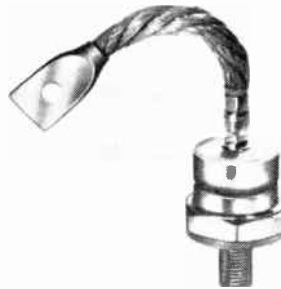
Silicon rectifier diode DO-8 has forward current capability up to 150 amps and prv ratings to 1,000 v. Freedom from thermal fatigue is achieved by use of a hard solder construction and matched thermal coefficients. The design utilizes the Solitron chip which features the hermetically sealed, glass passivated junction. Solitron Devices Inc., 256 Oak Tree Rd., Tappan, N.Y. [442]
