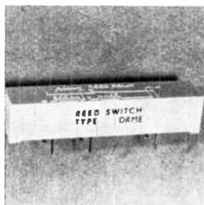
Dry reed relay type DRM features memory contact. Units are supplied with two coils, one to produce the make field, the other to produce the release field. Duration of energizing pulse can be between 10 μsec and steady d-c conditions. Average coil power is 250 mw for 6, 12, 24 v operation. Measuring Instrument Controls Inc., 438 Springfield Ave., Berkeley Heights, N.J. [343]
