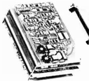
Four-microsecond random access memory system FI-2 is a 1024 word by 8 bit/word ferrite core assembly built on five interconnected circuit cards and designed to slide into a card cage or mounted remotely. Access time is 600 nsec. Power required is +12 v at 3 amps. Size 8 \frac{3}{8} x 4 \frac{7}{8} x 3 \frac{3}{8} in. North American Philips Co., Ferroxcube Systems Div., Englewood, Colo. [422]
