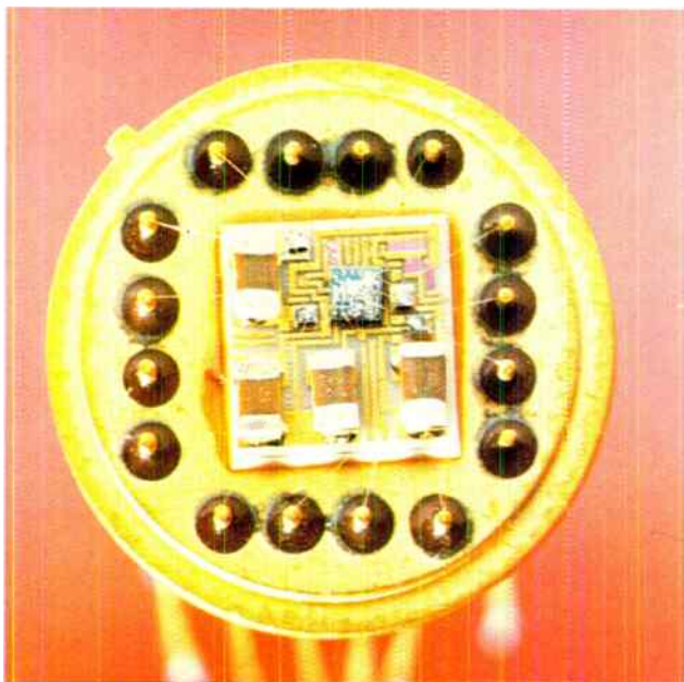
First . . . Chip and wire preamplifier with FET input is TI's first product in a new line of standard hybrid IC's.
