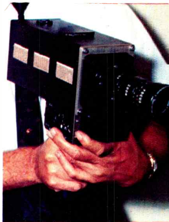
Spacebound. Westinghouse's color camera weighs a scant 15 pounds.
