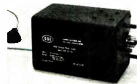
Power supply module HV-01-35 has multiple outputs of +12,000 \text{ v} , +400 \text{ v} and -100 \text{ v} available simultaneously. An internal voltage regulator allows operation of the supply from unfiltered d-c voltages between 35 and 50 v. Ripple is less than 0.1%. Temperature range is 0 to 50^\circ\text{C} . Price is $149.50. Sierra Systems Inc., 2255 Old Middlefield Way, Mountain View, Calif. [388]
