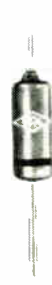
Temperature compensated reference diodes, with temperature coefficients as low as \pm 0.0005\% per° C, are available in JEDEC types 1N4565 through 1N4584A. They are designed to meet or exceed MIL-S-19500 requirements and can operate over a temperature range of -55° to +100° C. Centralab Semiconductor Division, 4501 N. Arden Dr., El Monte, Calif. [439]
