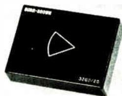
Wideband d-c operational amplifier 3260/25 has a guaranteed slew rate of 500 \text{ v}/\mu\text{sec} and settles to 1% of final value in 100 nsec. Rated output is \pm 10 \text{ v} , \pm 30 \text{ ma} . Open-loop gain is 80 db minimum. Unity gain bandwidth is 20 Mhz minimum. Voltage drift is \pm 25 \mu\text{v}/^\circ\text{C} maximum. Burr-Brown Research Corp., Int'l Airport Industrial Park, Tucson. [386]
