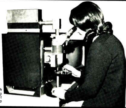
Basic LPM System with Universal Welding and Drilling Fixture and Closed-Circuit Television Setup
