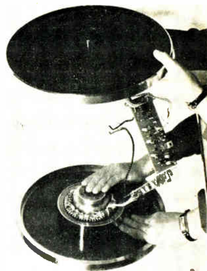
Direct. Turntable with transistor motor has no idlers, belts or pulleys. Its rotor is fixed directly to the turntable.
