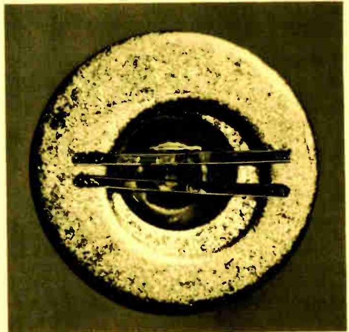
Construction of tuning varactor junction.
