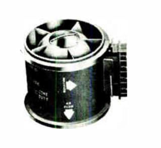
Small, lightweight vaneaxial fan Aximax 1 will provide 12 to 23 cfm at motor speeds between 11,400 and 22,500 rpm when operating at frequencies of 400 hz and above. The unit can also be supplied with a 60 hz motor that will deliver 3 cfm at 3,340 rpm. The airflow-reversible fan measures 1 1/2 x 1 3/4 inches and weighs 4 ounces. Rotron Inc., Hasbrouck Lane, Woodstock, N.Y. [347]
