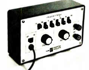
Compact digital pulse generator PG610 provides output pulses at repetition rates from 10 hz to 2 Mhz in six overlapping ranges. Output is compatible with TTL, DTL and RTL logic levels. It can be operated at high output pulse duty cycle. Dimensions are 2 x 3.75 x 6.25 in. Price (4-9) is $98.60. Computer Products, 2801 E. Oakland Park Blvd., Fort Lauderdale, Fla. 33306. [368]
