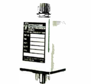
The TNR series is a solid state time delay (delay on energization) with dpdt relay output, 10 amp resistive at 115 v a-c. It is available with input voltage from 12 v d-c to 230 v a-c and in time ranges from 0.1 to 480 sec. Unit features reset during the timing period without any false transfer of output contacts. Syracuse Electronics Corp., Box 566, Syracuse, N.Y. 13201. [342]
