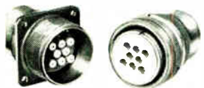
Eight-contact high voltage connectors in a standard MS type shell feature interfacial seals for each contact providing corona suppression through air excluding engagement. They are suited for high altitude applications to 70,000 ft and temperatures as low as -55°F. Silicone rubber inserts are supplied for normal use. Caton Industries Inc., 648 W. First Ave., Roselle, N.J. [345]
