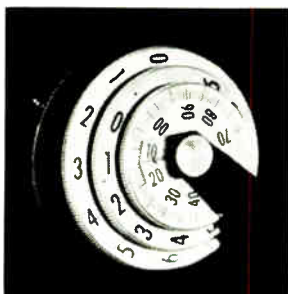
Tiny decade potentiometer designated DP310 Dekapot is a stacked-decade, coaxial-dial voltage divider. Professional grade components are assembled in the Kelvin-Varley circuit to provide terminal linearity of 50 ppm, high resolution (0.0035%) and constant input impedance. Price is $100. Electro Scientific Industries Inc., N.W. Science Park Dr., Portland, Ore. 97229. [341]
