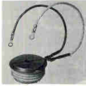
Full capacity thyristor type 282, designed to replace parallel scr's, permits upgrading of equipment with a minimum of external protection. When the device is water cooled, its rms current is 850 amps. Turn-on time is typically 5 \mu sec. I^2T is 200,000 amps squared seconds, and forward and reverse voltages range up to 1,500 v. Westinghouse Semiconductor, Youngwood, Pa. [437]
