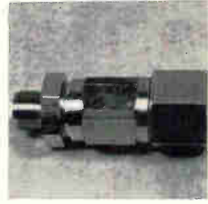
High voltage connectors series KV are less than 1 inch in diameter and will withstand 30 kv in a mated or unmated condition. They are available for various cable sizes—both flexible and semi-rigid—up through 3 inches. The connectors offer a pulse reflection coefficient of less than 1% maximum. General RF Fittings, Connector Division, Cove Road, Port Salerno, Fla. 33492. [344]
