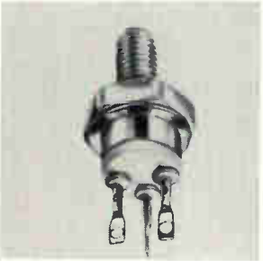
Isolated-collector, stud-mounted silicon transistors 2N5346-9 are medium-power npn devices with minimum f_T 's of 30 Mhz. V_{CEO} ranges from 80 to 100 v. Minimum beta at a collector current of 2 amps ranges from 30 to 60. Units are housed in a TO-59 package. Prices are between $24 and $34.95 in quantities of 100. Motorola Semiconductor Products Inc., Box 20924, Phoenix. [440]
