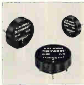
Distributed constant, fixed delay lines called Spiradel are compact and encapsulated for maximum environmental protection. Time delay to rise time ratios of over 20 to 1 can be achieved, with excellent temperature stability and pulse fidelity. Units cover a delay range of 100 to 1,000 nsec. Standard impedance is 325 ohms \pm 10\% . Allen Avionics Inc., E. 2nd St., Mineola, N.Y. [342]
