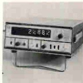
Counter/timer model 1605, for general lab and shop use, measures frequency from d-c to 25 Mhz. Features include input signal conditioning, gate times from 10 msec to 10 sec, 5-digit display with storage and automatic decimal positioning and an internal crystal oscillator with stability of 1 part in 10 8 /month. Eldorado Electronics, 601 Chalomar Rd., Concord, Calif. [368]
