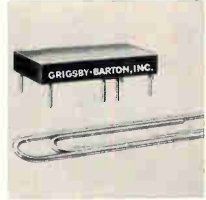
Compact reed relay GB811, in a 14-pin dual-in-line package, is completely compatible with IC logic components and p-c board pin spacing. Input is 5 v d-c for direct transistor logic drive, with the package containing both a reed relay and a diode to suppress back emf. Unit has a contact rating of 3 w. Grigsby-Barton Inc., 107 N. Hickory, Arlington Heights, Ill. 60004. [348]
