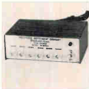
Crystal controlled frequency source model SS400 provides precise synchronizing pulses at 200, 400, 800, 1600, and 9600 hz. Frequency stability and accuracy of 0.005% are achieved. Unit is designed for laboratory use to synchronize RC oscillators at these fixed frequencies. It is priced at $98 and available from stock. Polyphase Instrument Co., Bridgeport, Pa. [363]
