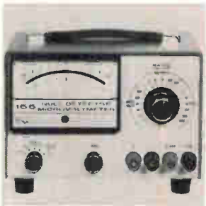
Combination null detector/micro-voltmeter model 155 offers 1 \mu v full scale sensitivity to 1000 v range. It features less than 150 nv noise, greater than 140 db common mode rejection ratio, and greater than 100 db normal mode rejection ratio, and greater than 10 12 ohms isolation from ground. Price (1-4) is $325 each. Keithley Instruments Inc., 28775 Aurora Rd., Cleveland. [367]
