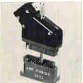
High density rectangular connector series HDR in 54-contact size features crimp-and-insert contacts on a 100-in. square grid pattern. Size 20 contacts are rated at 7.5 amps and come in two wire range sizes, 20-24 and 24-30 Awg. Contact plating is gold over nickel, selective gold, or tin. Housings are black phenolic or blue diallyl phthalate. AMP Inc., Harrisburg, Pa. [345]
