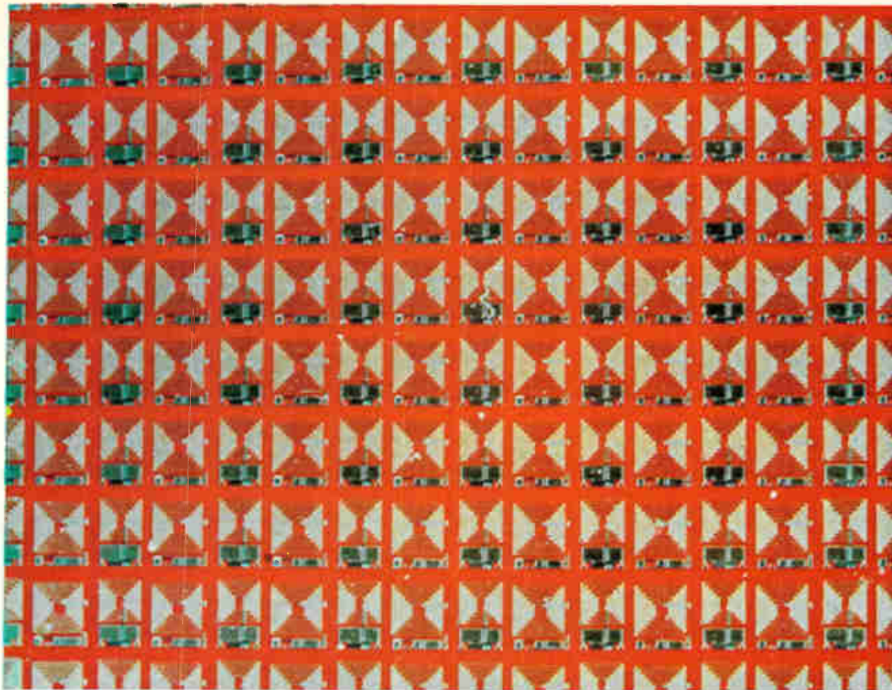
Lumped and batched. Passive elements of a 1-watt, 400-Mhz amplifier can be batch processed. Some 160 circuits fit on a 1-inch-square substrate.
