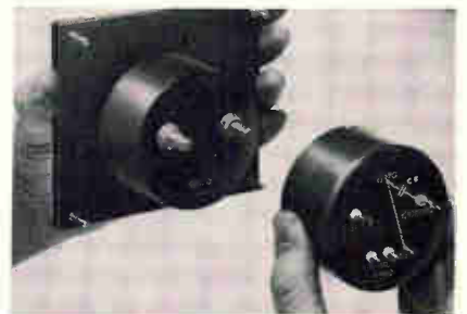
A joiner. The amplifier allows analog meter to measure a-c in the nanoamp region.
