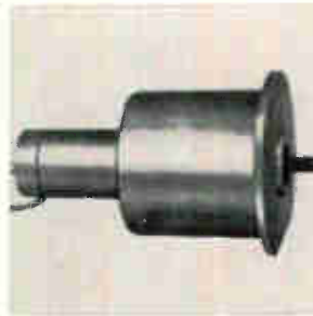
Servomotor tachometer size 23 is for use in power servo actuators. The 8-pole motor has a stall torque of 16 oz. in., and a free speed of 5,000 rpm. The tachometer produces an output of 2 v \pm 1\% per 1,000 rpm, has a phase shift of 0^{\circ} \pm 1^{\circ} , and linearity of \pm 7\% , and requires 5w of power. Operating temperature is -55^{\circ} to +132^{\circ} C. Weston-Transicoil, Worcester, Pa. [347]
