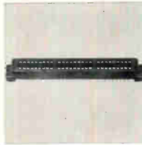
P-c connector series 600-121-27 is a 27-dual contact unit (54 terminals) with 0.100 in. center-to-center contact spacing. A choice of dip solder or solder lug terminations is available in gold plated beryllium copper. Glass reinforced diallyl phthalate molding type GDI-30 per MIL-P-19833 has 3 integral polarizing barriers. Continental Connector Corp., Woodside, N.Y. [343]
