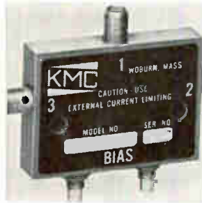
Thirty miniature diode switches, which occupy less than 3/4 cu. in. (excluding connectors) and operate over frequency ranges from 50 to 12,000 Mhz, are available. They provide switching speeds of 10 nsec from 2 to 12 Ghz, with power handling capability of 100 w peak and 1 w average. Typical dimensions are 1 3/4 x 1 3/4 x 1/2 in. Kevlin Mfg. Co., 26 Conn St., Woburn, Mass. 01801. [407]
