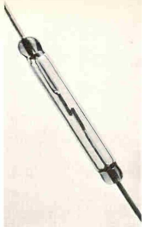
Slider. Twisted reeds slide along each other, keep contacts clean.
