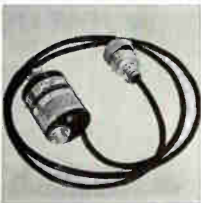
Coaxial, thin-film thermoelectric power heads models N420C, -21C, -22C and -23 operate from 2 Mhz to 12.4 Ghz. Vswr is a maximum of 1.5 over the entire operating range. They can be used with all the manufacturer's power meters. Each meter is capable of direct-reading power measurements from 30 nw to 3 w. General Microwave Corp., 155 Marine St., Farmingdale, N.Y. [405]
