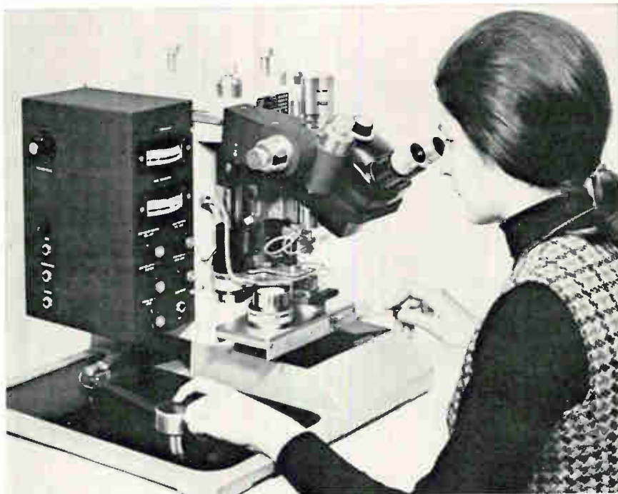
Leading off. Automatic bonders for beam-lead circuits, like this one from Kulicke & Soffa, are just now becoming commercially available.
