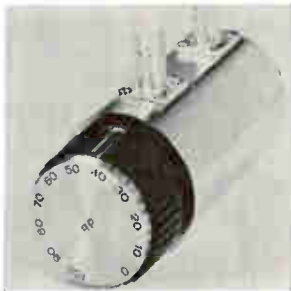
Rotary attenuator RA-100 covers 0 to 100 db in 10-db steps. It covers the frequency range of d-c to 1.2 Ghz with a 1.2:1 maximum vswr at 1 Ghz, with impedance of 50 ohms. The unit measures 1 7/8 x 2 1/8 in. Connectors available include the BNC, TNC, type N and STM. Price is $140 each with delivery in 2 weeks. Texscan Corp., 2446 Shadeland Ave., Indianapolis 46219. [406]
