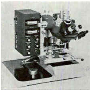
Semiconductor output is boosted by precision beam lead bonder model 573. Bonding is achieved by a thermocompression wobble tool and is readily adaptable to semiautomatic setups. A reflex optical system gives the operator a clear view of the device pattern superimposed directly on the workpiece pattern. Kulicke and Soffa Industries Inc., Fort Washington, Pa. 19034. [427]
