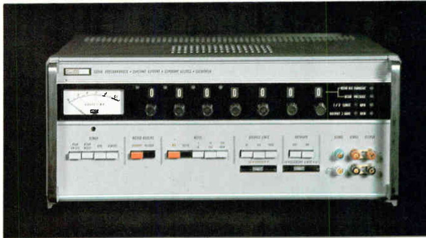
Steady I or V. The 3330A calibrator provides a programmable constant current or constant voltage and operates in automatic systems.
