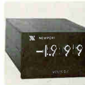
Digital panel meters 200, 210, 220 and 230 measure d-c voltage, d-c current, a-c voltage and a-c current, respectively, with full-scale display of 1,999 counts. Currents are measured from 1 na to 200 ma, and voltages from 10 \mu v to 200 v. Thirty-one different models and 13 options permit a variety of applications. Newport Laboratories Inc., 630 E. Young St., Santa Ana, Calif. [368]
