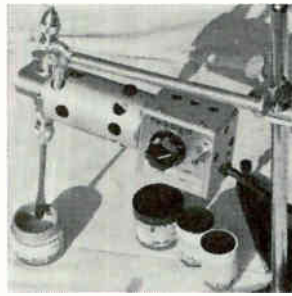
Paste power stirrer CM-6 handles emulsions, resins, and other thixotropic materials used in electronic fabrication. It features high torque and low speed. Continuously variable (between 0 and 1,000 rpm), the unit permits reproducible and uniform treatments to be applied to inks used in print and fire processes. Starnetics Co., 10639 Riverside Dr., N. Hollywood, Calif. [422]
