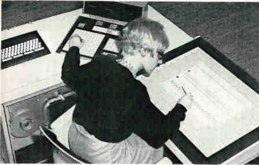
Quick on the draw. Telefunken's graphics-input terminal converts sketches to digital data that a computer can process. An ordinary ballpoint pen or sharp pencil will work on the 18-by-24-inch input pad.
