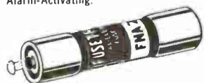
FNA FUSETRON Fuse 13 32 x 1 1/2 in. slow-blowing, Visual-Indicating, Alarm-Activating. (Also useful for protection of small motors, solenoids, transformers in machine tool industry.)
