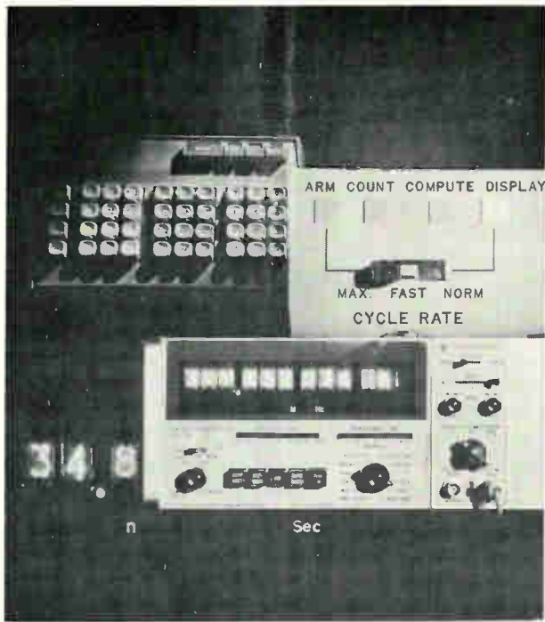
It counts; it figures. Hewlett-Packard's newest entrant in the counter timer race is the 5360A which, is both a fast and accurate counter and a calculator.
