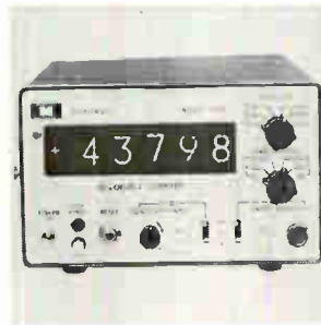
Reversible 2-channel counter model 106A has a 5 hz to 5 Mhz counting rate for each channel. Versatility is provided by the rapid counting rate, combined with averaging capability as well as measuring sum and differences. The unit measures 4\frac{3}{4} \times 7\frac{1}{2} \times 9 in., weighs 5.6 lbs. Price is $895; delivery, 4 weeks. Monsanto Electronic Instruments, 620 Passaic Ave., West Caldwell, N.J. [363]
