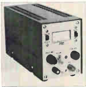
Constant voltage, constant current lab power supply QAD50-1 has 0.01% regulation. It is designed for applications such as computer controlled lab testing requiring programing either up or down at a rate of 10 mv/ \mu sec. Ripple is less than 0.5 mv rms or 2 mv peak-to-peak with excellent stability. Price is $99. Todd Products Corp., 28 Laurel St., Hicksville, N.Y. 11801. [382]
