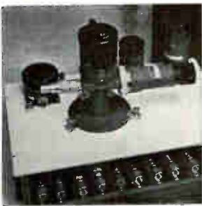
Standing wave detector type 2219K measures vswr and angle of reflection coefficient over a frequency range of 10 to 2,300 MHz at a sensitivity of 5 mw. It eliminates heavy slotted sections and features adapters to all standard coaxial transmission lines. Detector components are now available in a kit form. PRD Electronics Inc., 1200 Prospect Ave., Westbury, N.Y. [401]
