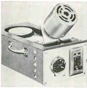
Wavedipper WD-4-HT "RR" solders at temperatures up to 850° F. It is for such applications as soldering relay coil bobbins using polyurethane insulated wire. Special treatment of its tank and pump prevents intermolecular migration between tin-lead solders and stainless steel parts that usually occur at higher temperatures. Electrovert Inc., Hartford Ave., Mt. Vernon, N.Y. [421]
