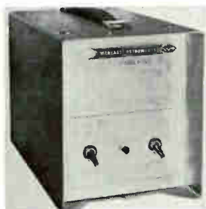
Scope pack model P-TEK improves the performance of oscilloscopes and crt devices. It provides 50 db filtering to 1 Mhz and 0.25% regulation. Scope problems such as pretriggering, jumping off scale, false signals, jitter, and erroneous readings caused by line disturbances are virtually eliminated. Price is $325. Wanlass Instruments, 1540 E. Edinger Ave., Santa Ana, Calif. [361]
