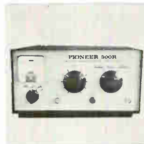
Secondary frequency standard 300R can be used in the receive mode for calibrating oscillators directly without the use of an oscilloscope or other indicating device. Stability is 0.005% (5 hz at 10 khz, 0.01 hz at 200 hz). A switch selects up to 3 standard frequencies. Price is $169.50; availability, 4 weeks. Pioneer Electronics, 738 Pacific St., San Luis Obispo, Calif. [367]
