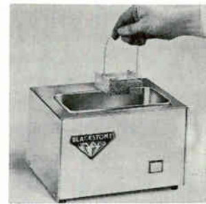
Portable ultrasonic cleaner model SP-100 measures 10 5/8 x 8 1/2 x 6 3/4 in. and incorporates a stainless steel tank with a capacity of 1 3/8 quarts. Its 100-watt average output results in high intensity uniform action and efficient cleaning in the removal of grease or contaminants. The unit's only control is an off-on switch. Blackstone Ultrasonics Inc., Sheffield, Pa. 16347. [424]
