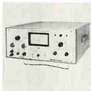
A-c/d-c transfer standard model ATS converts rms to d-c at 0.01% accuracy in 15 seconds. It converts a d-c digital voltmeter, potentiometer, or any d-c measuring system to a true rms measuring system. Its rated accuracy covers the range of 0.25 to 1,000 v and 5 khz to 20 khz. Price is $3,500; availability, from stock. Singer Co., 915 Pembroke St., Bridgeport, Conn. 06608. [366]
