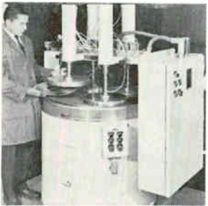
Free-abrasive machinery tool is for semiautomatic controlled-temperature polishing of memory disks used in the computer field. Designed to polish 4 disks simultaneously, the machine features automatic timing, a vacuum system that holds the memory disk to the chuck, and a continuously rotating polishing wheel. Speed-Fam Corp., 509 N. Third Ave., Des Plaines, Ill. 60016. [425]
