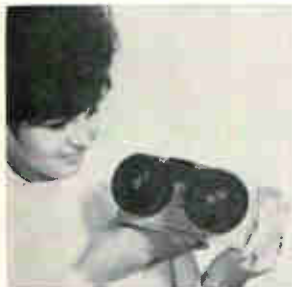
Bulkhead-mounted, single line punched tape reader model 3100 is designed for loading computers, controlling test equipment, and similar uses where a small tough unit is required. It will withstand 2 g vibration from 5 to 33 hz, and 25 g shock. Operating temperature is -40^{\circ} to +70^{\circ} C. Price is $1,190. Electronic Engineering Co. of California, E. Chestnut Ave., Santa Ana, Calif. [425]
