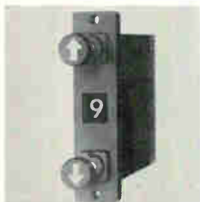
Bidirectional push-button rotary switch called Space-Saver comes in 8, 10, or 12 positions in all standard codes. Life characteristics include 100,000 cycles (a cycle consists of 720° rotation). It carries 3 amps continuous, makes and breaks 0.125 amp resistive at 28 v d-c and 115 v a-c, 0.05 amp inductive at 28 v d-c. Janco Corp., 3111 Winona Ave., Burbank, Calif. [341]
