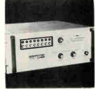
Analog-to-digital converter model HS-810 will assign up to 10 million 8-bit binary numbers/sec to wideband analog signal. Codes available are straight or offset binary, 1's or 2's complement, or Gray. It has a maximum error of 0.2% \pm ½ least significant bit and a maximum aperture time of 0.4 nsec. Computer Labs, 1109 Valley Park Dr., Greensboro, N.C. 27403. [428]
