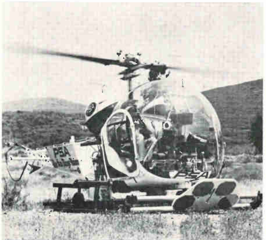
Where are you? Direction-finding gear developed by Cubic Corp. can home in on SOS signal at distances of 2½ miles through dense, wet jungle. The range of conventional gear is limited to a mile.
