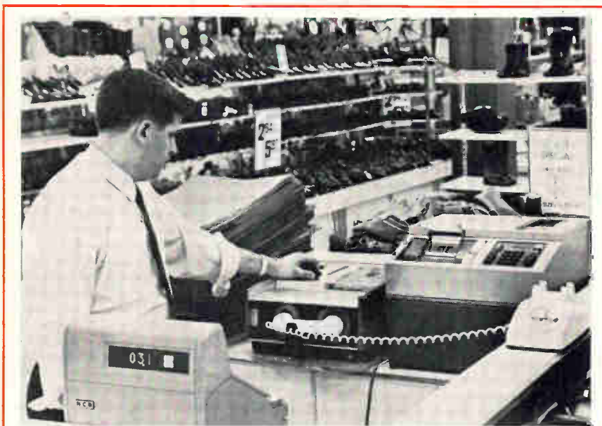
Point of purchase. Up-to-the-minute inventory figures can be calculated with this system, developed by the Kimball Systems division of Litton Industries. When a clerk rings up a sale, he feeds the punched price tag into the machine, which then stores the data collected from the tag. Later the machine transmits the data by telephone to a central computer.
