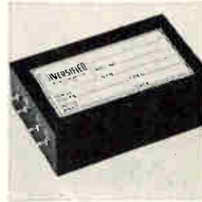
Active bandpass filters series DE500 with integral detector cover the 1 Hz to 10 kHz frequency range. Out-of-band rejection is greater than 60 db. Input signal is 1 to 5 v rms. Input impedance is 600 ohms. Operating voltage is 12 to 15 v d-c at 100 ma. Size is 1 x 2 x 3 inches. Price is less than $150. Diversified Electronics Co., 154 San Lazaro Ave., Sunnyvale, Calif. 94086. [344]
