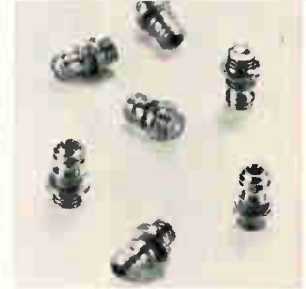
C-w avalanche oscillator diodes series MA-4900 are designed to accomplish a one-step conversion from d-c to microwave energy, thereby eliminating complex circuitry. Typical performance is represented by the MA-4980 which operates over the 8.2 to 12.4 Ghz range with minimum output of 10 mw and efficiency of 1 to 2%. Microwave Associates, Burlington, Mass. [443]
