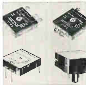
Solid state relay SSA withstands extreme environmental conditions of shock, vibration, heat and acceleration. It offers a predictable threshold voltage for pull-in and drop-out. The contacts always close when a minimum of 3 v is applied to the coil, and will always open when applied voltage is reduced to less than 3 v. Ohmite Mfg. Co., 3601 Howard St., Skokie, Ill. [342]
