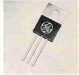
Six-ampere SC141 and ten-ampere SC146 plastic triacs have applications in control circuits for major appliances. They feature a molded gray silicone package, round leads for easy handling and mounting, a solid copper heat sink for low thermal impedance (2° C/w), and a glass passivated triac pellet insuring hermeticity. General Electric Co., 1 River Road, Schenectady, N.Y. [439]
