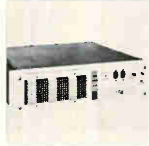
Programmable data comparator series 800 provides monitoring of up to 100 points, with point scanning frequency of 200 khz. Programming is sequential, requiring only a single advance signal input to move from point to point. Data word length is 4 BCD digits, plus signal. Peak-to-peak amplitude of input signals is 10 v max. Systems Research Corp., 2309 Pontius Ave., Los Angeles. [427]
