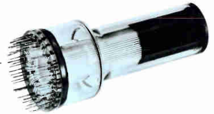
Mosaic. A lead selenide 56-element detector array, made by Santa Barbara Research Center, packaged in a Dewar.
