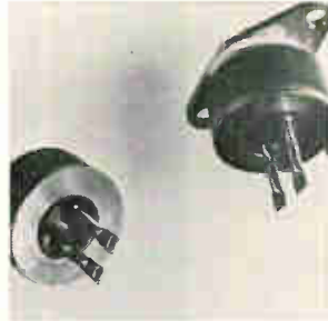
Solid state relay R160, a replacement for electromechanical relays, combines semiconductor and IC technology. Packaged in a 3/4-inch press-fit case, it is available for actuating voltages of 6, 12, and 24 v d-c at a gating current of 35 ma. The unit will control a power circuit of 16 amps rms at 120 v, 50 or 60 hz. Hunt Electronics, 2617 Andjon Drive, Dallas 75220. [441]
