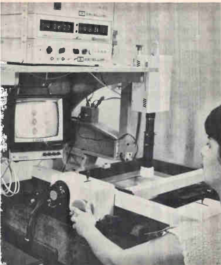
Tape by tv. An artwork master on tv is used to prepare a control tape for the drilling machine.
