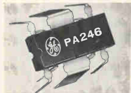
Same form. The package of the 5-watt amplifier is the same size as the 2-watt version (top). Two large heat-sink tabs replace the single sword-shaped one.
