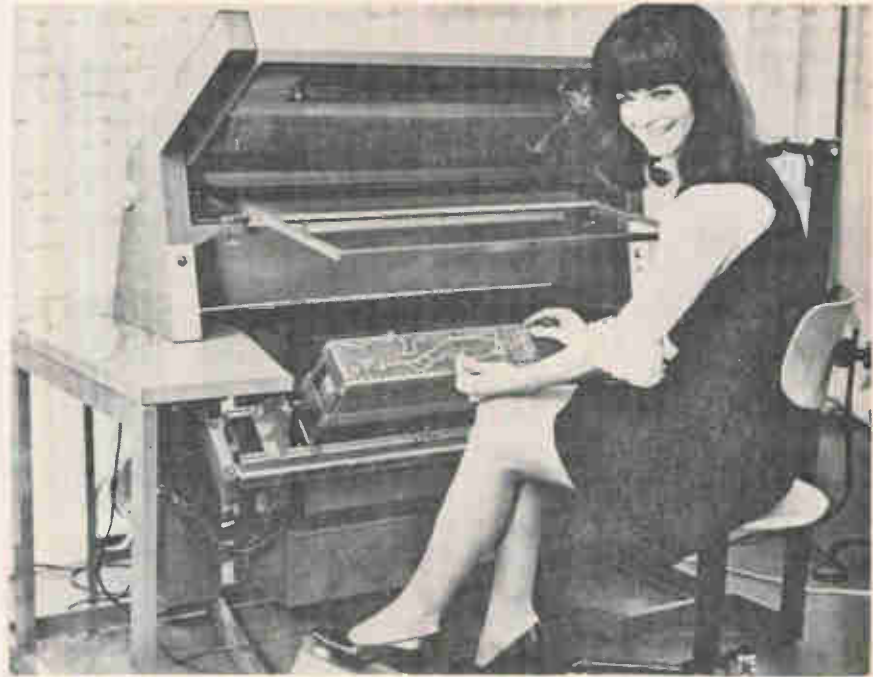
Light work. AEG-Telefunken's semiautomatic wiring equipment has connection tool that won't go on to next step if all isn't well.
