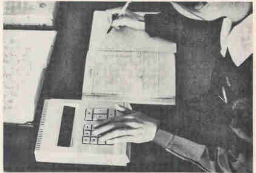
Summing up. This miniaturized experimental desk calculator was developed by Hayakawa and uses large-scale integration [Electronics, Nov. 11, p. 307]. It contains 11 MOS integrated circuits with 300 to 400 elements each, three bipolar hybrid IC's four bipolar transistors.
