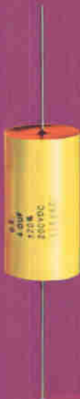
Polycarbonate Tubular Capacitors (left) 64 standard ratings. 100 and 200 volts d-c, 0.001 to 1.0 \mu f, -55 to 85C
