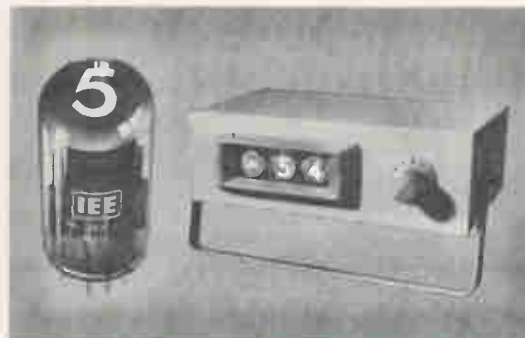
nimo™ —First 10-gun CRT single-plane display. Projects numbers, letters and words onto a fluorescent screen. No image ambiguity. No external focusing required. No ambient light worries. Exceptionally wide viewing angle. Ideal for instrument application.
