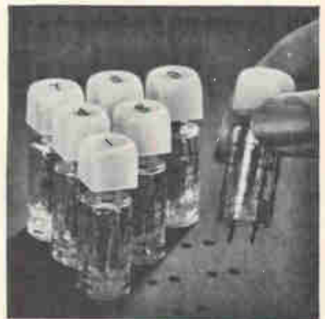
Simple, low-cost mounting. Raytheon switches plug into .125" PC board. Contact pins snap in, firmly lock switch in place for soldering. This permits you to use flow soldering techniques—cut keyboard assembly time and costs.
