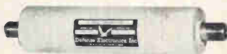
TPA-70 and TPA-73 S and L-Band Preamplifiers. S-band: 6 db. Maximum noise: 20 db. Minimum Gain/ L-Band: 5 db. Maximum Noise: 20 db. Minimum Gain/ No Parametric Oscillation with Signal Overloads/ High immunity to strong signal burnouts/ Power output for 1 db Amplitude Compression: -5 db minimum.
