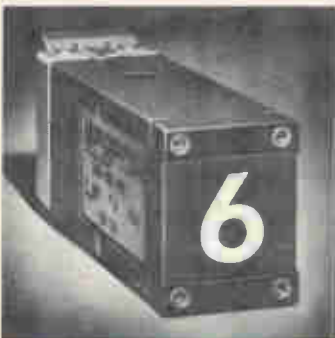
120H —Miniature rear-projection readout (.62" sq. screen) easily read from 30' under high ambient light. Quick-disconnect lamp assembly speeds lamp replacement.
