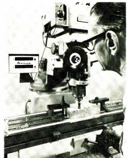
Where it's at. As table moves, output pulse-rate of transducer changes.
