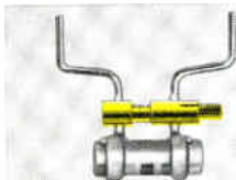
Solder ends to terminals of another component.
