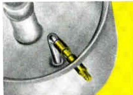
Solder one end to coupling link and other end to cavity wall.
