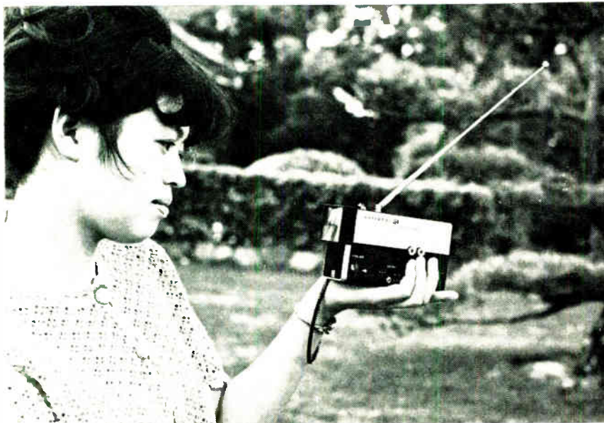
Video on the go. Matsushita's 2-in. black-and-white television set plays two hours between battery changes.
