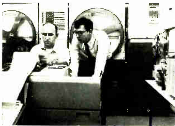
Updating. Test technician and programmer use keyboard to write test programs for new devices or to update programs in the memory. Typewriter printout can be used to record data on the devices being tested.
