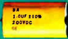
Metallized Film Flattened Oval Capacitors 102 standard ratings, 100 and 200 volts d-c, 0.01 to 10.0 \mu f, -55 to 85C
