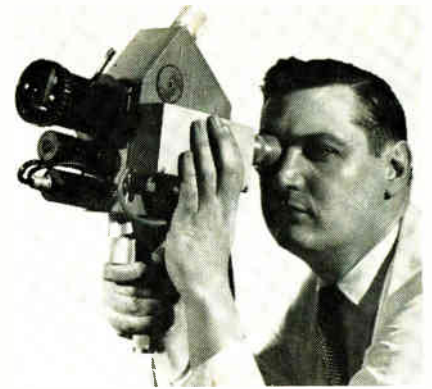
Mighty mite. Experimental portable color tv camera built by Norelco uses 5/8-inch Plumbicon tubes.
