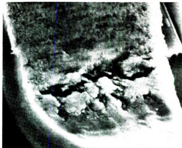
Blowup. Scientists at NASA's Electronics Research Center used a scanning electron microscope to look at aluminum leads ultrasonically bonded to an IC pad. They discovered these transverse microcracks, shown magnified 2,300 times.
