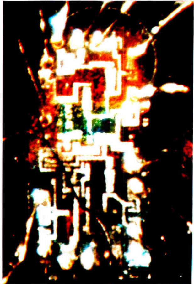
Crystal detector. Hot spots on IC's can be detected with liquid crystals. In the IC above, the hot spot is the blue resistor-diode circuit. The heat dissipation across the IC's surface is shown by the color change from blue to red. The coating, supplied by Liquid Crystal Industries, changes color with minute changes in temperature.
