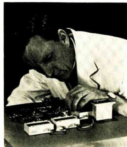
Viewpoint. Engineer checks broadband parametric amplifier built by Northern Electric for satellite ground station.
