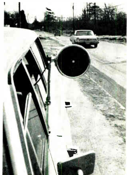
Pull over. Varian's Bomac division has developed an impatt diode as the microwave power source for police radar traps. Solid state device shrinks system into two packages—meter and controls, on the left, and antenna, right. But its price—still a few hundred dollars more than conventional gear—is keeping it out of the market. One design is being tested by the Mini Quip Corp.
