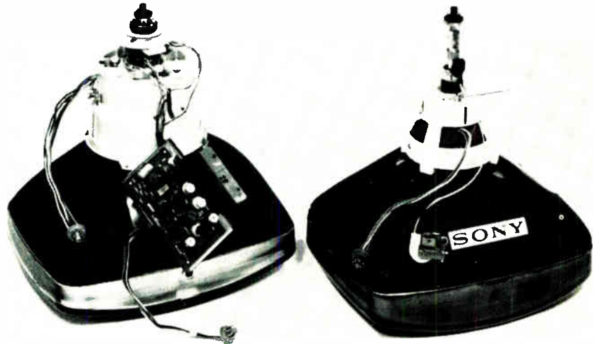
Yoke-less. With the Trinitron gun, Sony's tube needs no convergence yoke and panel. Flyback, shown resting on tube, does the job.
