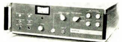
Booster. Power amplifier supplies 1 watt minimum from 1 to 12.4 Ghz.
