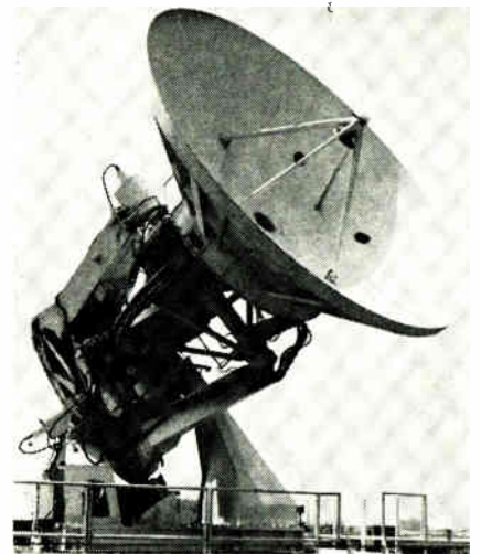
Looking up. Millimeter-wave antennas are being used to predict sun spots.
