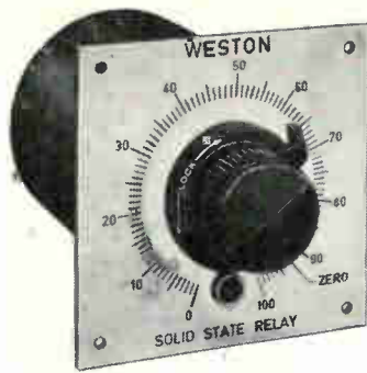
Model 1062 Control Relay—no moving parts, not even relay contacts; voltage ranges from 0-1 volt, current ranges from 0-100 \mu a; 200-millisecond response time with 0.5% repeatability typical; zero adjust and trip indicator on 320° scale.
