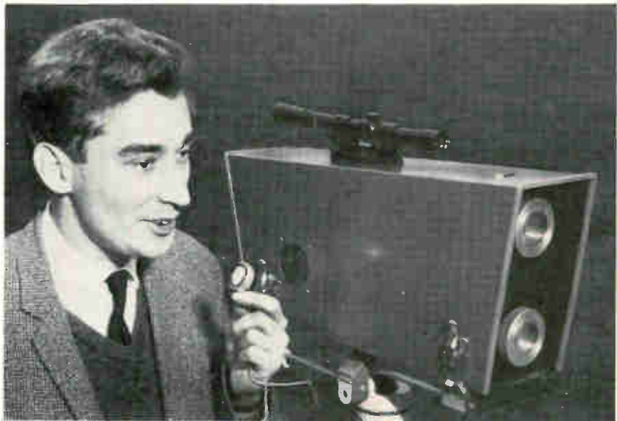
Rig with a yig. Mullard's Roger Cooper talks over infrared telephone link built around the magneto-optic modulator he developed.
