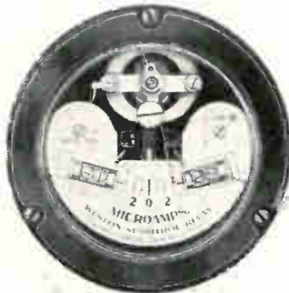
Model 723 Sensitrol® Relay—sealed; shielded; internal reset; solder terminals; single or double magnetic contact; ranges as low as 1-0-1 \mu a.
