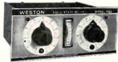
Model 1066 Dual Set-Point Relay—with input monitor and independently adjustable set points. Repeatability \pm 1/2\% ; accuracy \pm 2\% ; selectivity to 1 \mu a; switching capacity 1 amp at 117 volts AC.
