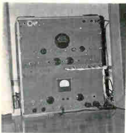
Stop and go. Reverberation generator delays audio inputs, avoids distortion.
