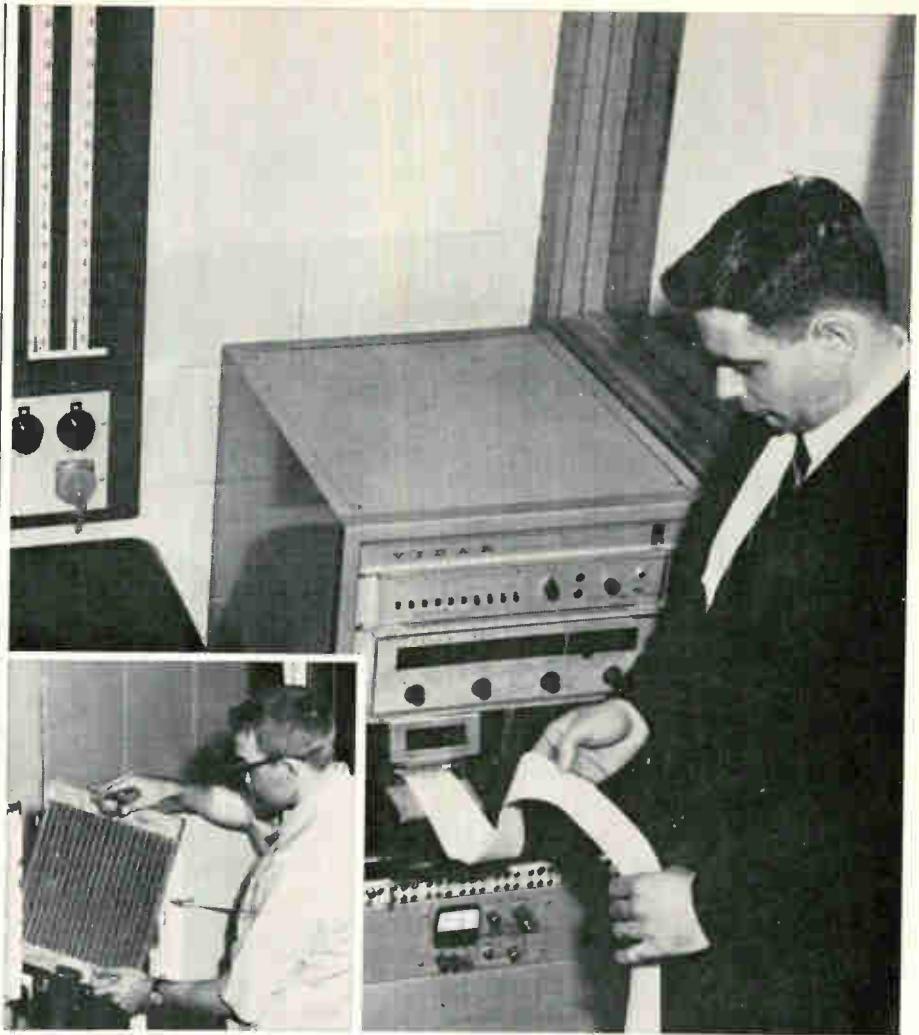
Modine technician prepares test core for wind-tunnel test. VIDAR Digital Data Acquisition System speeds testing of automotive and industrial radiators, oil coolers, and other related products.
