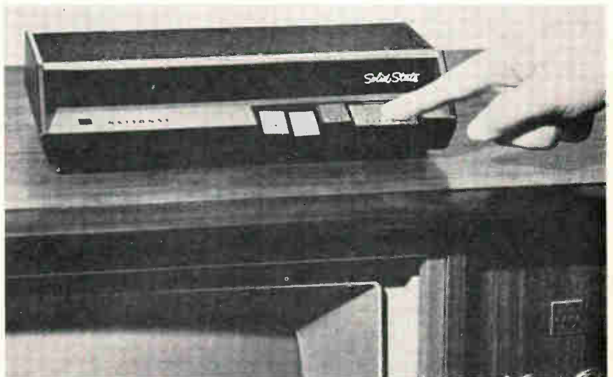
Step by step. Varactor diodes in Matsushita's uhf tv tuner provide key to channel selection as in vhf band. Other uhf tuners have variable capacitors and, therefore, continuous tuning.
