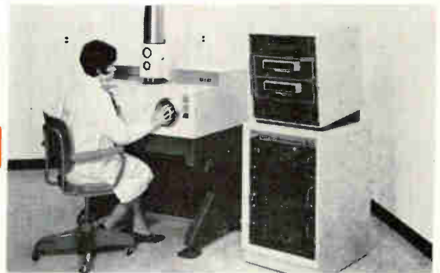
Reduced artwork is master for step-and-repeat camera.
