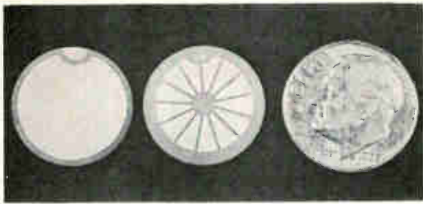
Ferroelectric pie. Costing only about a dollar, this little wafer can store a number and transfer it directly into an electronic counter. A voltage applied to the bottom layer bends it; the upper layer bends too, generating voltage pulses at the pie-shaped electrodes. Pulse polarity depends on previous polarization of the ceramic.
