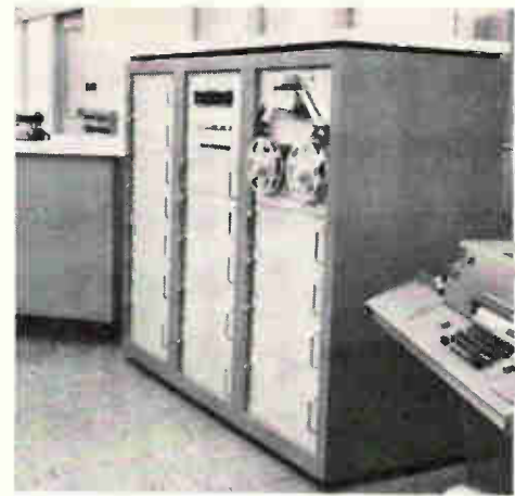
Prober. Machine is designed to test as many as 3000 terminals at a time.
