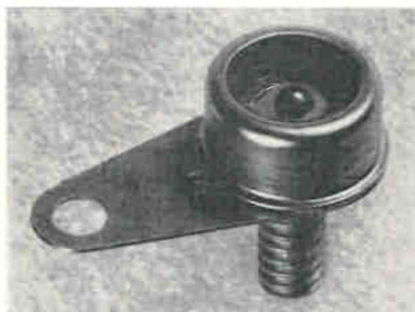
Well-rounded. Light-emitting diode made with hemispherical dome to improve light emission properties.
