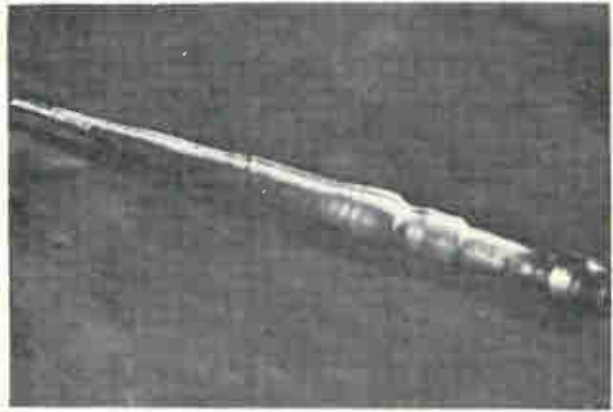
Czochralski crystal. Cylindrical shape results from twisting as crystal is lifted from the melt.
