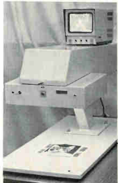
Still life. Pickup unit of Philips' system that transmits still photos, drawings and the like during the vertical blanking periods of regular tv broadcasts.
