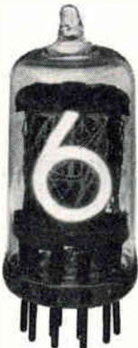
8754—Also available with right- and/or left-hand decimal points; Interchangeable with NL840/8754. Decimal-point types interchangeable with NL841, 842, 848.
