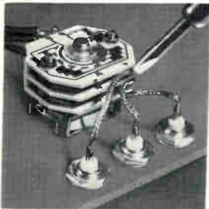
Switch plus. Wafer can have as many as 10 resistors screened on each side.
