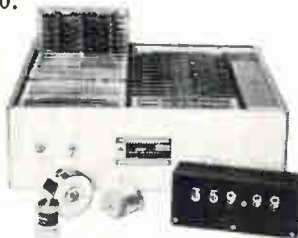
Figure 3. Model 5450 Automatic Angle Position Indicator. It measures shaft angles, converts them to digital data.
