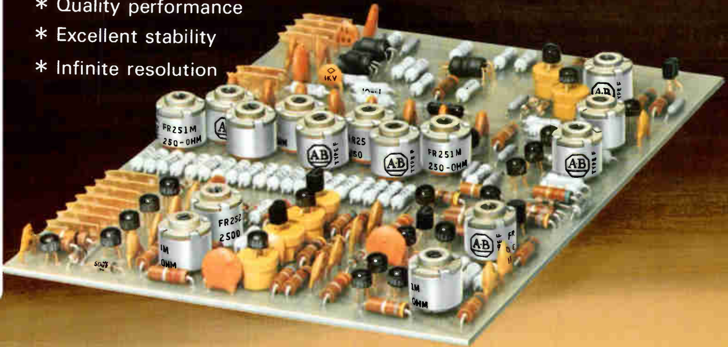
One of the 5-inch by 6½-inch Wavetek printed circuit cards, showing 15 of the 25 Allen-Bradley Type F hot molded variable resistors and numerous hot molded fixed resistors used in the Model 111 VCG function generator.
