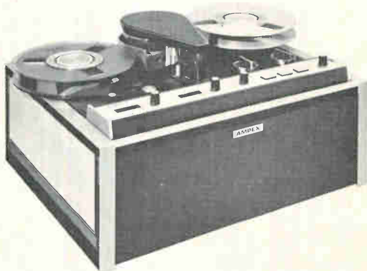
For the record. Ampex VR-5000 tape unit, smallest in the company's line, weighs 64 pounds, can be used with any standard monitor or television set.
