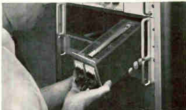
You can mount up to 4 units in a standard LRA-1 or LRA-2 rack adapter.
