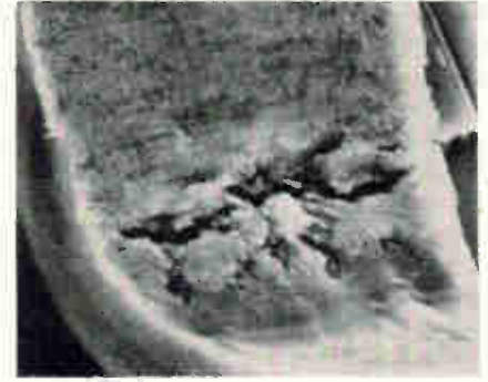
Flaw. Scanning electron microscope at 1,000 × magnification (left) and 3,500 × discloses fault in gold lead ultrasonically bonded to gold pad. This fault would not be detectable by optical methods.
