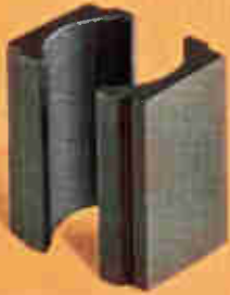
A-B ceramic magnets used in the 500 Selektronic shaver shown actual size.
