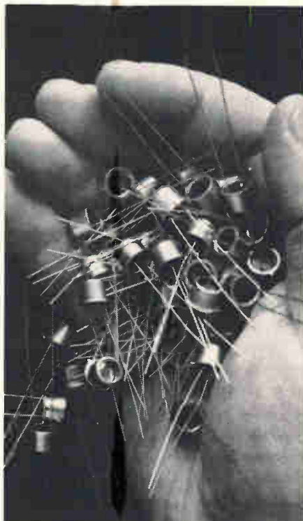
Array. Developmental array of light-emitting diodes is a step toward solid state alphanumeric displays.
