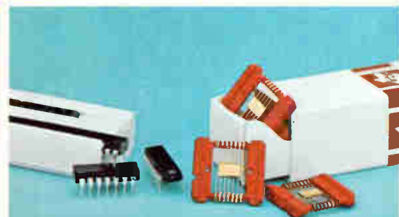
Series 54H/74H offered in both dual-in-line and flat packages
