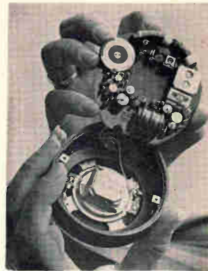
Handful. Philips portable boasts a pair of integrated circuits and snug packaging.
