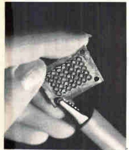
Array. Developmental array of light-emitting diodes is a step toward solid state alphanumeric displays.
