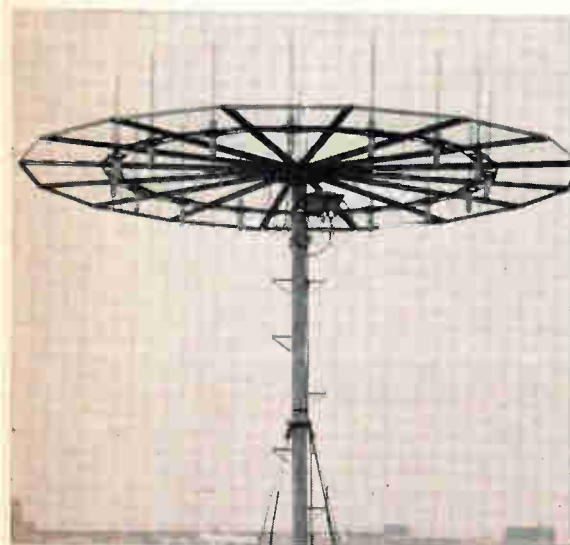
Plane spotter. Ring of monopole antenna elements picks up small aircraft's radio transmission and from it determines plane's bearing.
