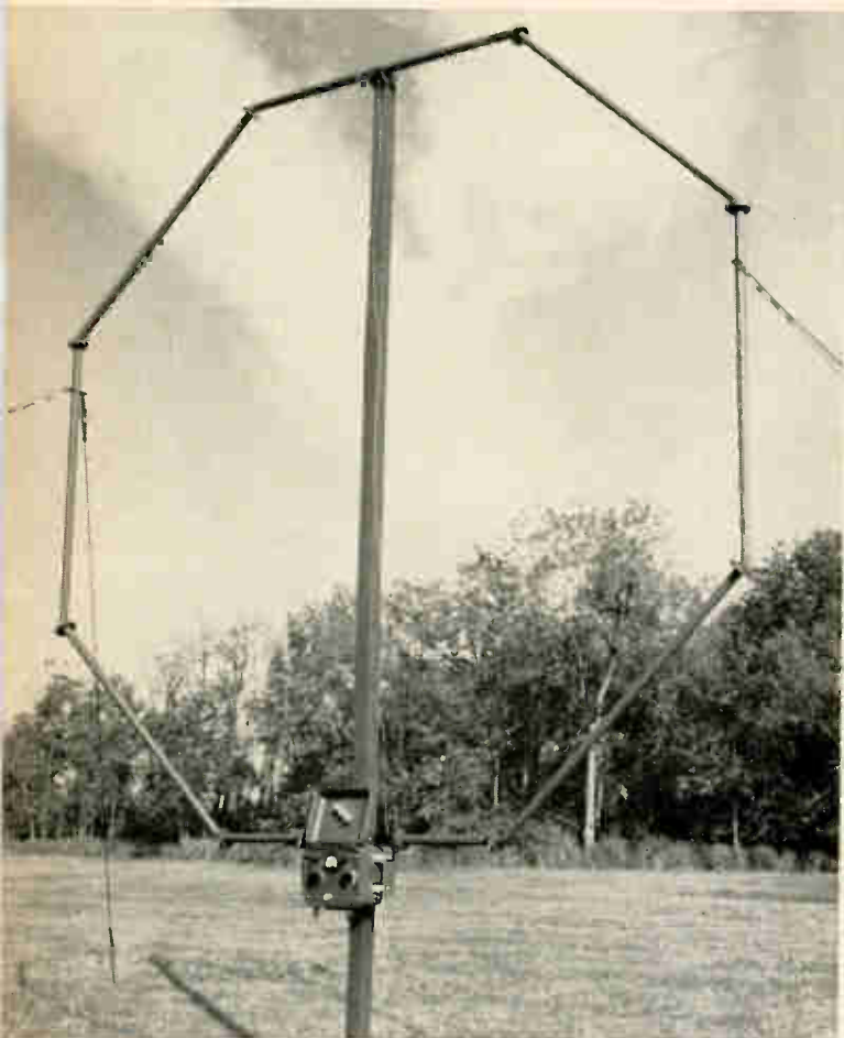
Will travel. Octagonal loop antenna with 5-foot sides is easily set up, dismantled, and transported. Efficiency near the earth matches that of conventional elevated antennas as long as several hundred feet.
