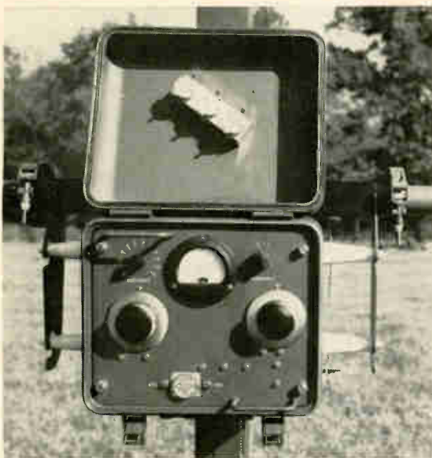
Precise tuning. Reflected power meter permits fine tuning and exact matching, and monitors forward output power level. The coarse adjustments make discrete, step-by-step changes, while the fine controls provide continuous variations overlapping the coarse steps.
