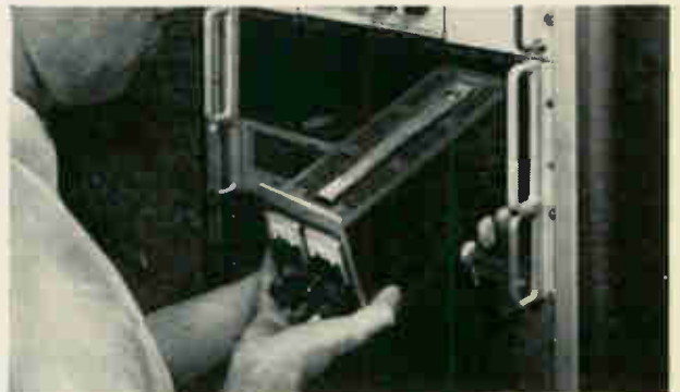
You can mount up to 4 units in a standard LRA-1 or LRA-2 rack adapter.
