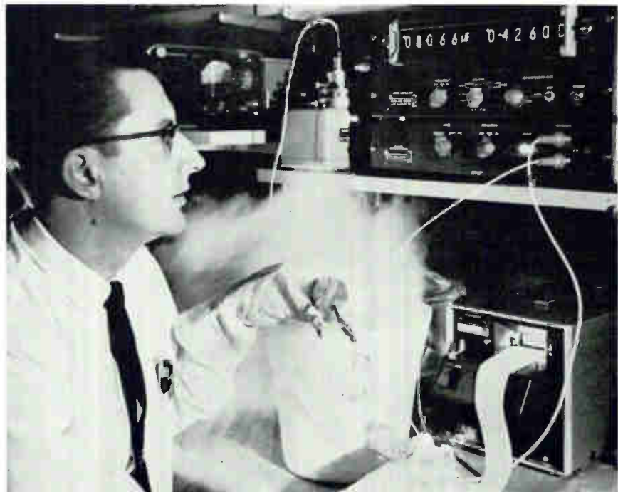
Down cold. General Radio's automatic capacitance bridge permits faster cryogenic tests than are possible with conventional instrumentation.
