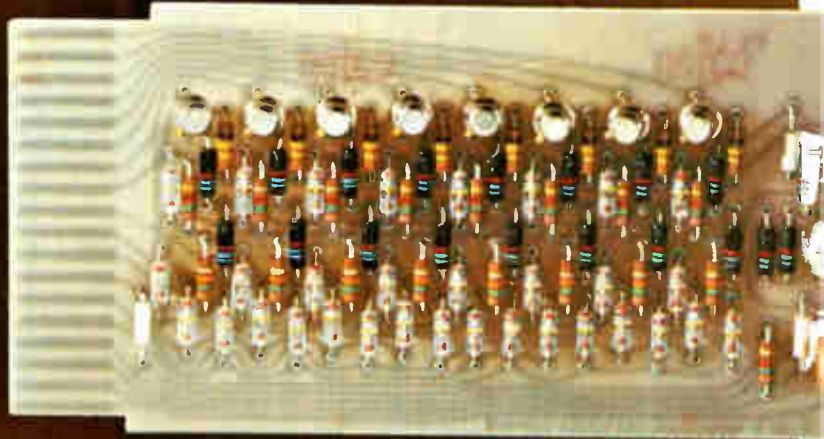
FLIP CHIP T.M. Modules —The Digital Equipment Corporation trademark for a new kind of digital system module uses Allen-Bradley hot molded resistors exclusively.
