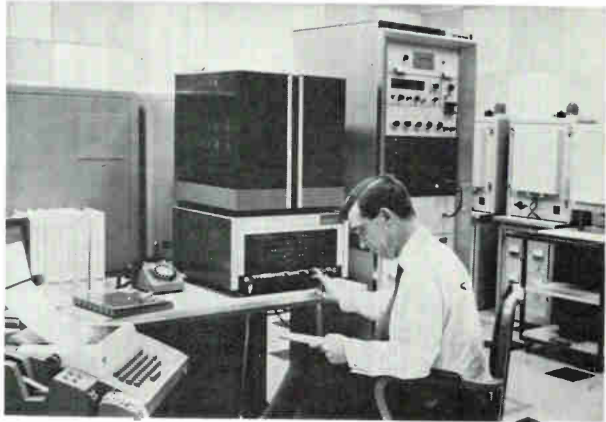
Components on trial for reliability characteristics are closely monitored and analyzed by computer in center of product test facility. Mounting frameworks for thin-film circuit modules are attached to the doors of test chambers at right.
