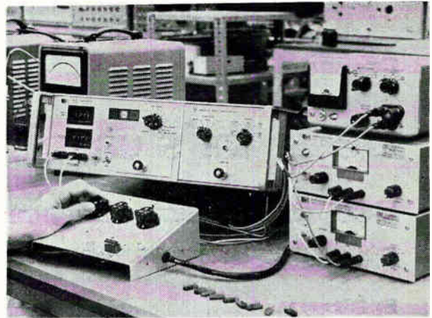
Limit comparator can be used with external test jig for integrated circuits.
