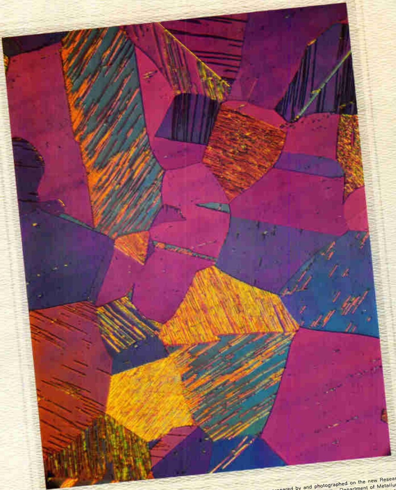
Specimen: Austenite (6% manganese, 1% carbon, 93% iron). Rolled, quenched in brine from 2000°F. Etched with Vilella's reagent. Original magnification: 100X.
