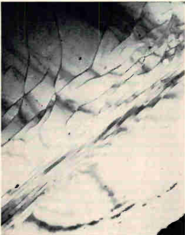
Dislocation structure, discontinuities on surface, are shown magnified with an electron microscope. The dislocation is at the surface of a power transistor near the junction region. Such a fault could lead to a soft junction and to abnormal electrical properties in the IC.
