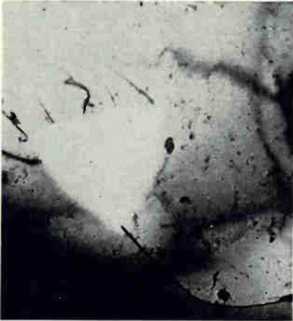
Transmission electron micrograph shows both a triangular and linear defect in the base region of a device. Such defects can lead to shorts or opens, or even cause parameters to drift. The device is magnified 5,000 times.
