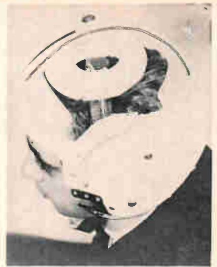
Experimental microphone built into top of helicopter crewman's helmet enables him to talk without interference from wind noise and to keep both hands free.
