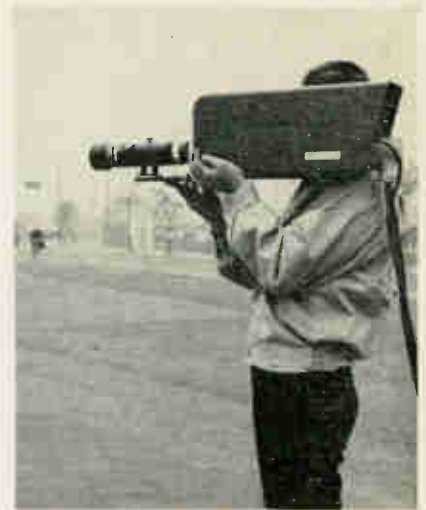
Single-tube color tv camera developed by Nippon Columbia Co. registers blue and red chrominance information as black-and-white stripes.
