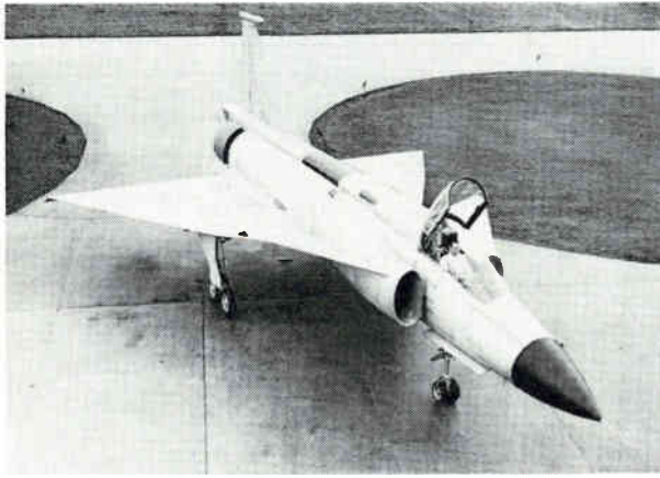
Future mainstay for Swedish military-electronics producers is the Saab 37-Viggen, Sweden's next generation supersonic interceptor-reconnaissance aircraft. Its initial flight will come early this year.
