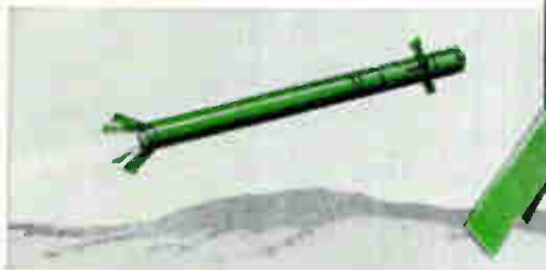
Infrared sensor locks on target. Miniature computer directs steering fins to guide Redeye.
