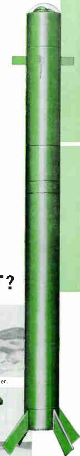
Infrared sensor locks on target. Miniature computer directs steering fins to guide Redeye.
