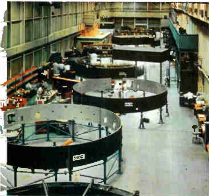
On a production line in a special plant in Huntsville, Ala., IBM turns out the ring-shaped instrumentation units that control the vehicle during takeoff.
