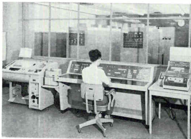
Central computer installation for JNR's seat reservation system.
