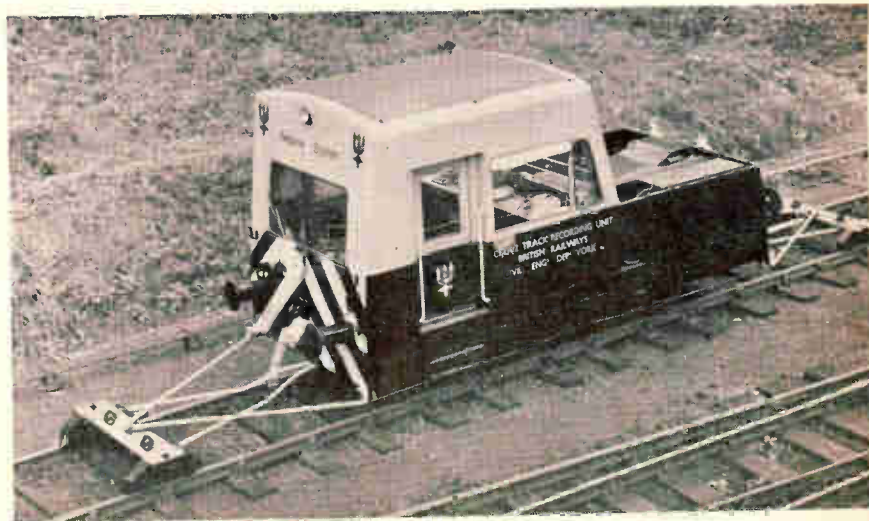
British Railways' Neptune system puts computer on track-checking trolley to spot faults quickly.
