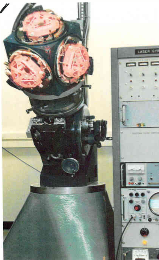
Three-axis laser gyro unit mounted on this test stand was delivered to the Navy for shipboard tests.
