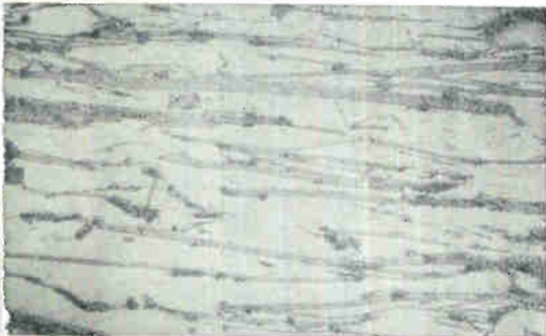
Layered structure of semiconducting glass-bonded mica, magnified 300X. Such high-strength composites can also be made with boron-nitride dielectric and graphite.
