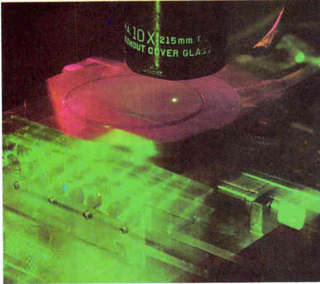
Many-circuited wafer is coated with photoresist, exposed in unique pattern by ultraviolet beam (bright spot).
