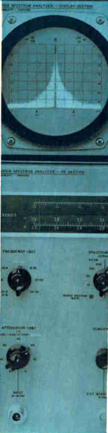
Radiation from an electric drill held next to the antenna is displayed by the spectrum analyzer and up-converter. Horizontal scale, 30 kHz/cm centered at 150 kHz; vertical scale, 10 dB/cm.
