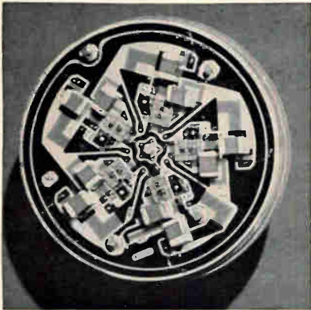
Eventually, each of the discrete component subassemblies in the synthesizer will be reduced to an IC similar to the one-inch diameter disk shown above. This is the first of the microminiature circuits that are being developed for this unit. It is part of the prescaler—a divide-by-5 stage.
