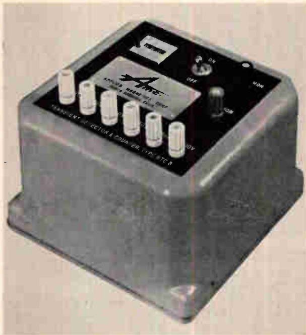
Detector-recorder is used for determining the transient level and frequency of occurrence. The data is needed in selecting the proper gap.
