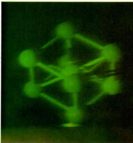
Model of molecule whose three-dimensional image has been reconstructed with ordinary white light. Hologram was made with laser light.
