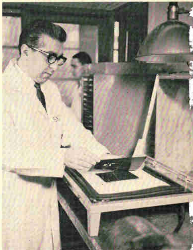
Reduced size negative is used to expose a light-sensitive coating on the copper clad dielectric. After spraying with a suitable etch, only sections of copper corresponding to the center conductor configuration will remain.
