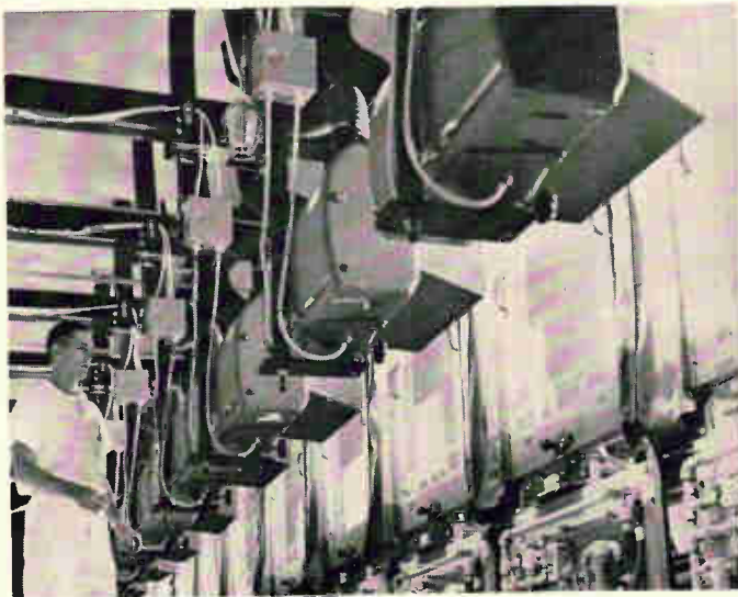
Production line for the manufacture of shadow masks, a key element in color television tubes.
