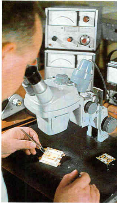
Bell's Paul Stark checks a 3.5- to 4.5-Gc hybrid IC during final assembly.
