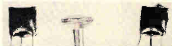
Mounting the silicon die on a small metal tab, attaching wire leads and encapsulating made the device smaller.
