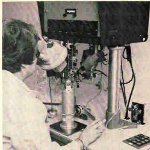
Ultrasonic bonder attaches gold leads to chip mounts and to thin-film conductors on the hybrid-circuit substrate. The close-up photograph at the left shows the bonding tip poised above a transistor mounted on a ceramic channel.
