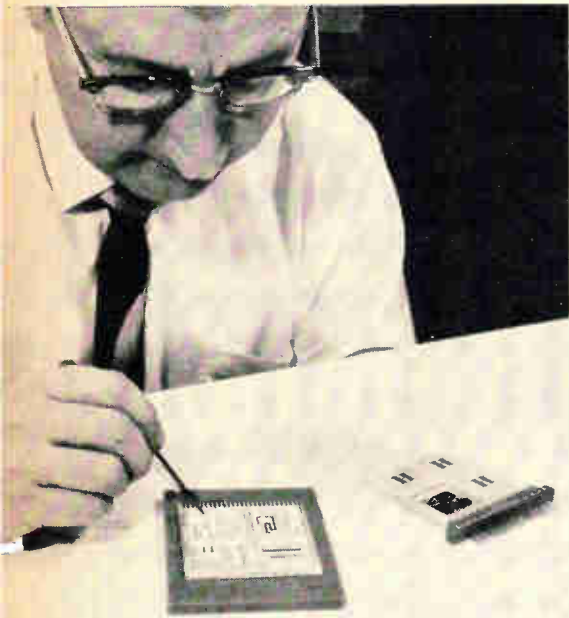
Modular hybrid-circuit array is built by sealing four ceramic frames to a ceramic base, putting thin-film circuits into the frames and then sealing the frames with ceramic covers. A base-frame assembly and an almost-completed array are seen in the photo. The circuits are interconnected with conductors (color, in drawing) that are screen-printed on the base along with power resistors and package leads.
