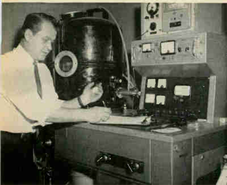
Research engineer Harry Bajars times the wafer metal bonding-layer deposition, accomplished by sputtering from a sheet cathode in a chamber containing argon.
