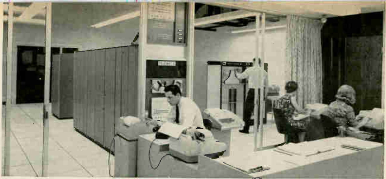
Massachusetts General Hospital's computer system for medical record-keeping and research. The computer, installed at Bolt Beranek & Newman Inc.'s laboratory in Cambridge, is about seven miles from the hospital. The computer can be seen immediately behind the operator's panel to the right of the man at the teleprinter. Behind the computer are the memory banks; in the extreme rear is one corner of the drum storage unit; tape drives are visible at the right.
