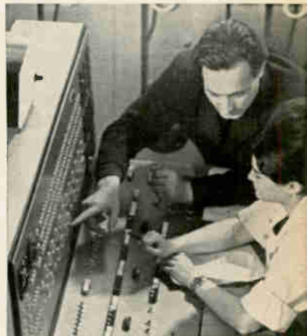
Minsk 22 is Russia's newest civilian computer. Its twin memory system has been called inefficient by Leningrad engineers, who modified it with a single memory block twice the size of either original memory. But production models still use twin memories.
