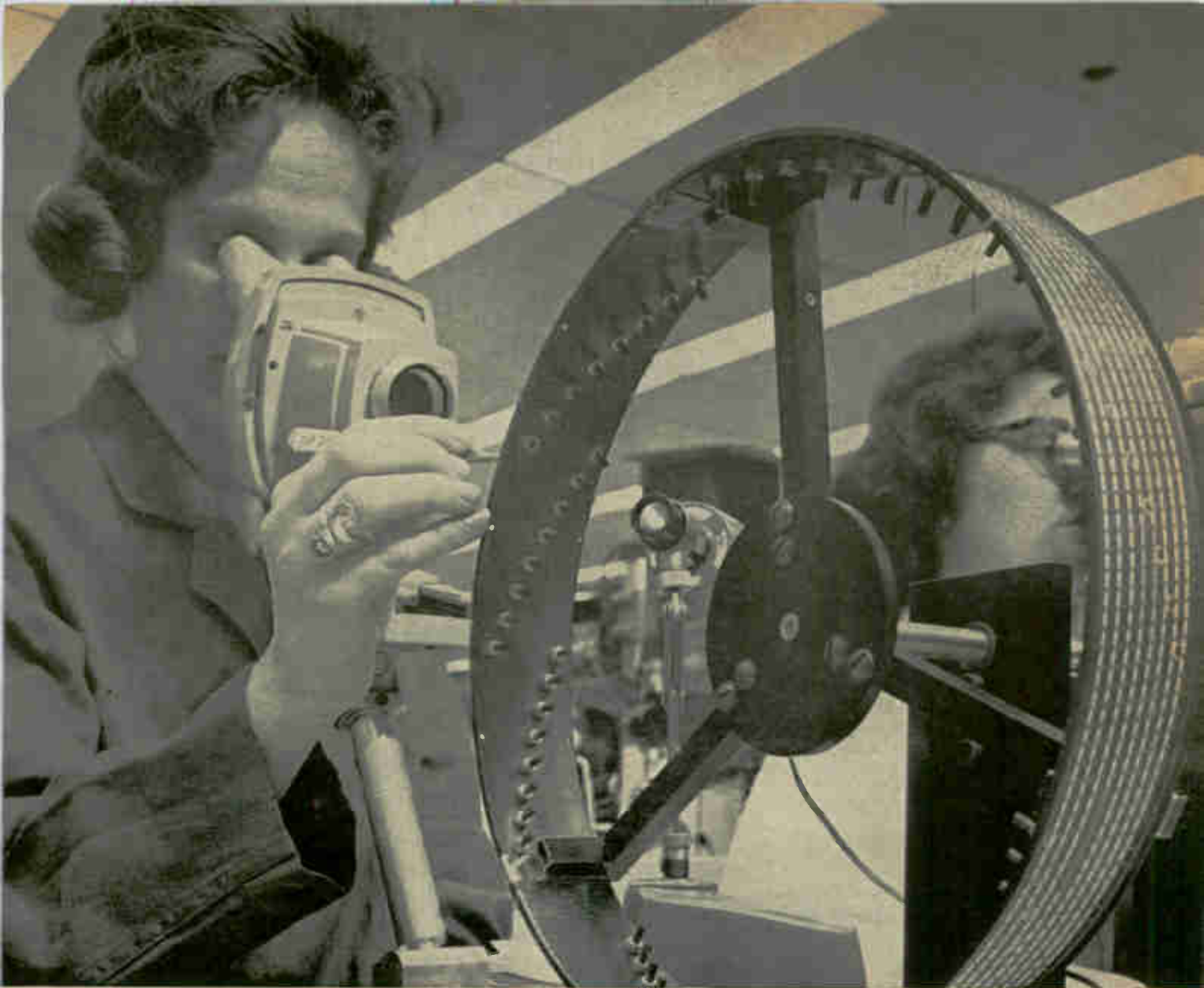
Magnetic drum carries more than 1,000 transistor chips on a single strip of Kovar foil. It loads and unloads production machines, is a processing fixture and, as shown above, makes visual inspection of unpackaged devices a rapid procedure. The little studs on the drum's inner circumference are ferrite magnets which hold the strip.
