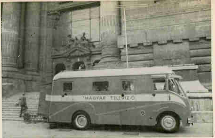
Mobile units, like this Hungarian van used for on-the-spot news coverage, transmit to the studio by microwave relay.
