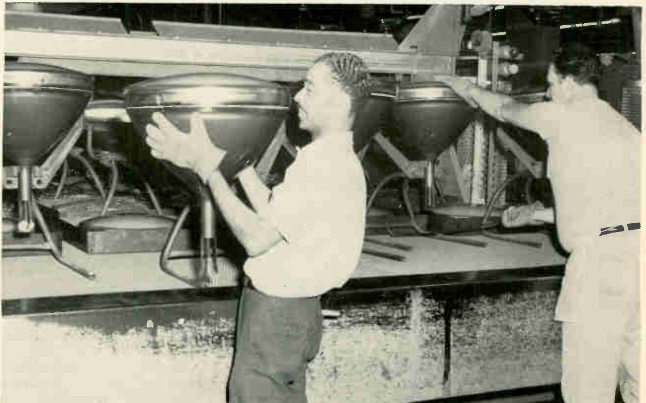
Color-tube assembly line at Philco's Lansdale division, after several months of production, is producing 2,000 tubes per week. Total production of color tubes from eight manufacturers will be over 4.5 million this year.
