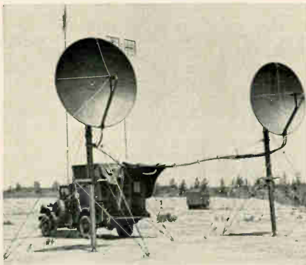
Tactical communications systems, like this AN/TRC-97, are being sought by the Pentagon to provide the military with "a little Bell System" on the battlefield.
