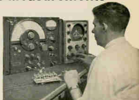
An experimental 5-stage, single-tuned, 30-Mc i-f strip with 1-Mc bandwidth being aligned with the Type 1025-A Standard Sweep-Frequency Generator. Data measured includes center frequency, 6- and 60-dB bandwidths, and gain. The generator can be accurately set to both the 10 \mu V signal level at the front end as well as to 100 mV at the last stage.
