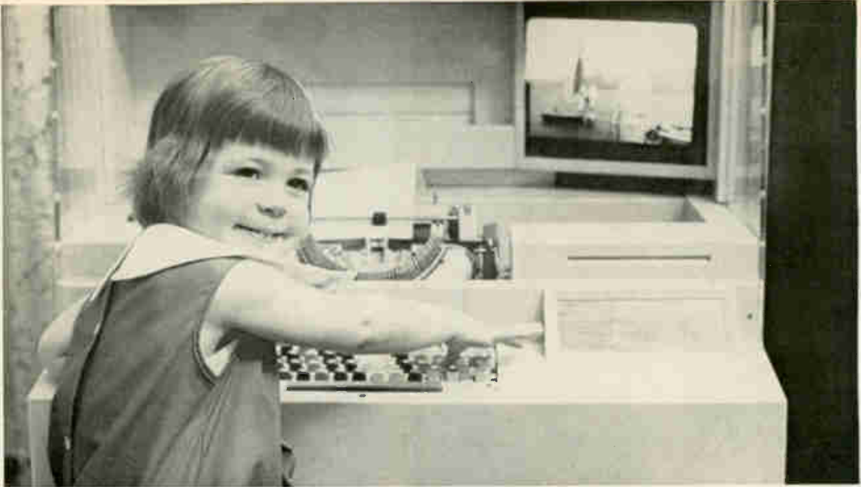
Called the talking typewriter, this machine, developed by the Edison Laboratory division of the McGraw-Edison Co., helped preschool children learn to read, write and touch-type. It contains computer-controlled keyboard, random-access audio storage and slide projector.
