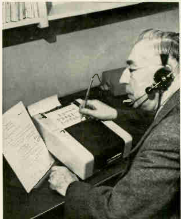
Lecturer Howard F. Fehr at Columbia University in New York speaks into headset while writing on an Electrowriter. Both voice and writing are carried by phone lines.
