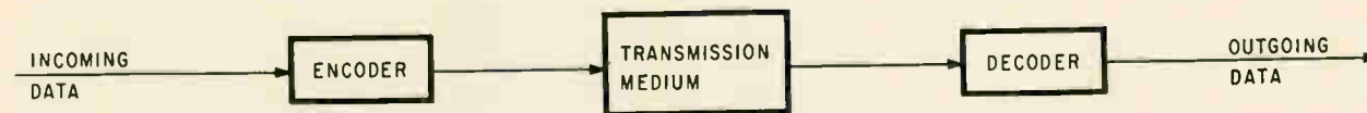
Forward-error-correction systems insert redundancy into the transmitted bit stream to correct errors. Greater code redundancy is required for error correction than for error detection.
