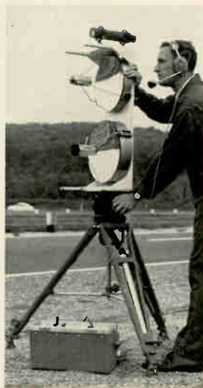
Optical communications system developed by David E. Wright, an engineer at Edgerton, Germeshausen & Grier, Inc. provides a low-cost voice link up to eight miles.
