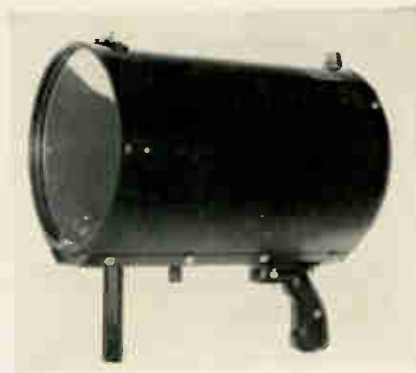
Hand-held optical communications unit converts voice signals into light pulses. Receiver reconverts the light into voice signals.
