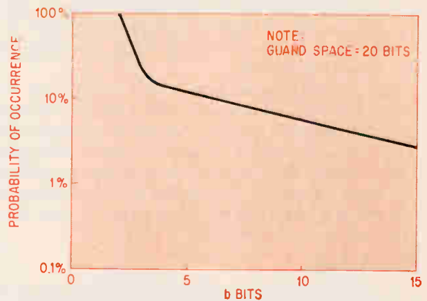
Measured statistical distribution of error-burst lengths, plotted as a function of a number of binary bits in the burst. The curve indicates that 90% of the error bursts last less than 7 bits.
