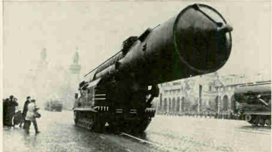
This Iron Maiden rocket, encased in a cylindrical pod, can be launched from its own self-propelled transport. Weapons paraded in Red Square showed Soviet emphasis on mobility and longer range. The Russians also displayed a 115-foot "orbital missile."
