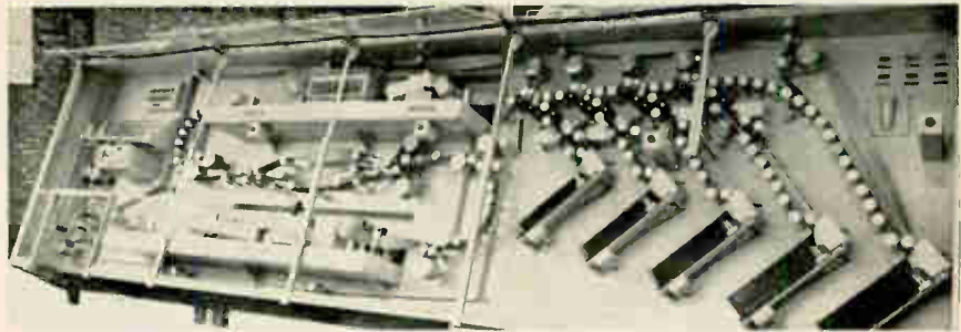
Mail handler consists of feed-in section at left, scanning shelves in center and stamp-canceling and letter-stacking unit at right. Conveyor belt carries letters from one section to another.
