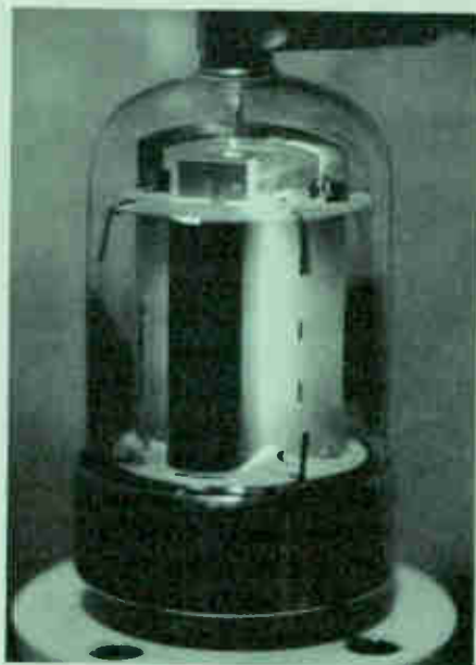
Unretouched photo of 6146B with conventional plate. Note pronounced hot spot.
