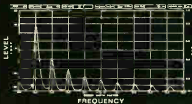
Harmonic contents of a complex waveform analyzed on the 12" x 4½" chart readout of the SY-1 Sonic Analysis System.
