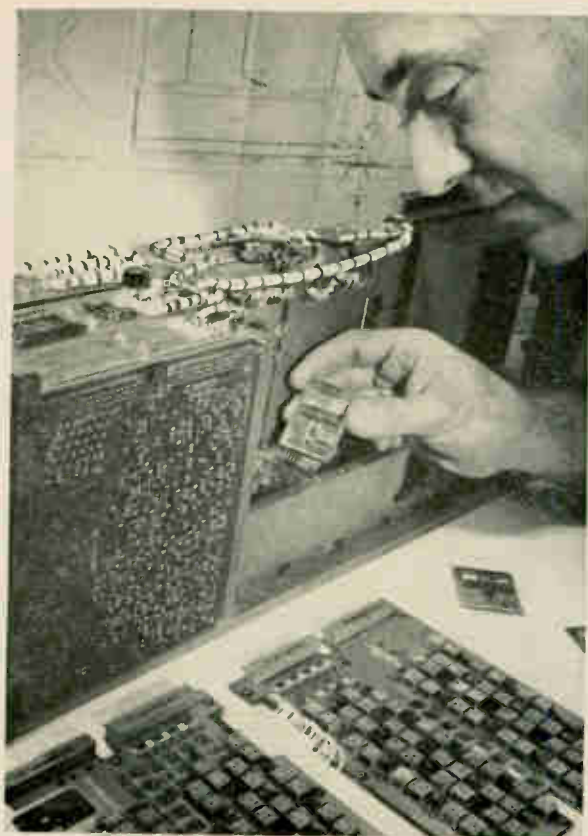
Monolithic and hybrid circuits are generally employed in the memories of new, small aerospace computers. At left, the memory of Honeywell, Inc.'s H-387 computer is being assembled. At right, a portion of the logic system is being put together. Multilayer boards are used to interconnect the logic circuits.
