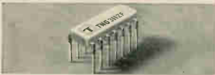
HLTTL Circuits available in this 14-lead plug-in package
