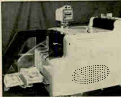
Yen counter employs electronic circuits to reject marred bills without stopping the machine.
