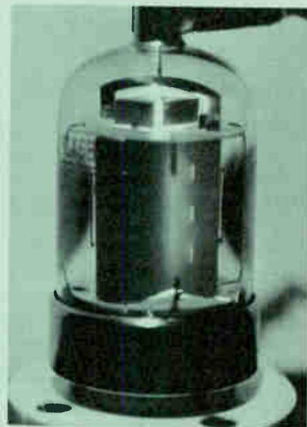
Unretouched photo of Sylvania 6146B with Hi-Con plate. Note absence of any color.
