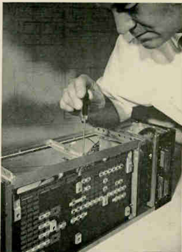
Monolithic and hybrid circuits are generally employed in the memories of new, small aerospace computers. At left, the memory of Honeywell, Inc.'s H-387 computer is being assembled. At right, a portion of the logic system is being put together. Multilayer boards are used to interconnect the logic circuits.
