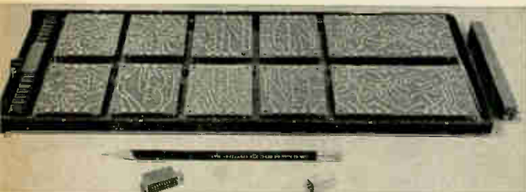
Mobidic computer's Level II assembly had six modules with one or two circuits per module. The small objects in front of the pencil are volumetric assemblies of equivalent function, used as Level I microelectronic modules.
